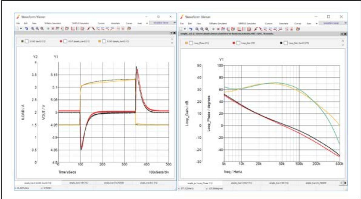
Figure 1. Both step-load transient response (left) and AC analysis Bode plots (right) show very good agreement between simulated vs. measured results for the MAX17244 synchronous buck converter. Lab data is shown in black ( $V_{OUT}$ , gain) and green (current step, phase), while simulated data is shown in red and orange.
