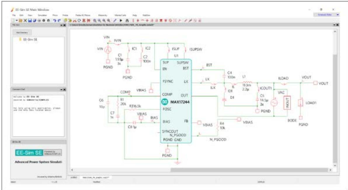
Figure 2. MAX17244 SIMPLIS synchronous buck converter schematic.
