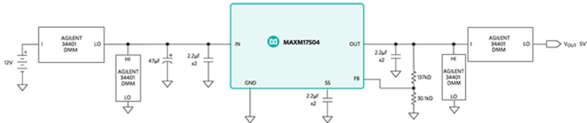
Figure 3. Efficiency measurement circuit using 4 DMMs.
