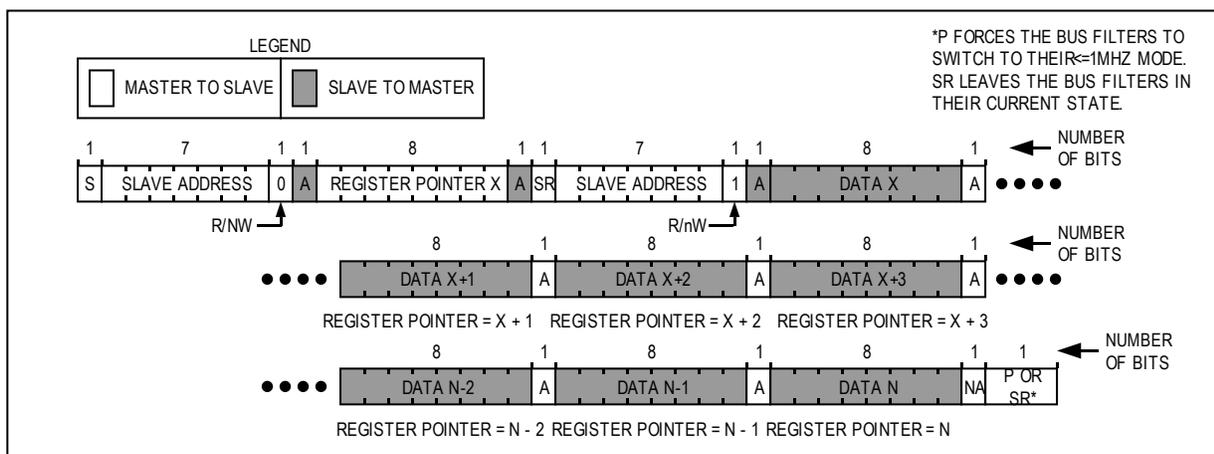
Figure 8. Reading from multiple registers.
