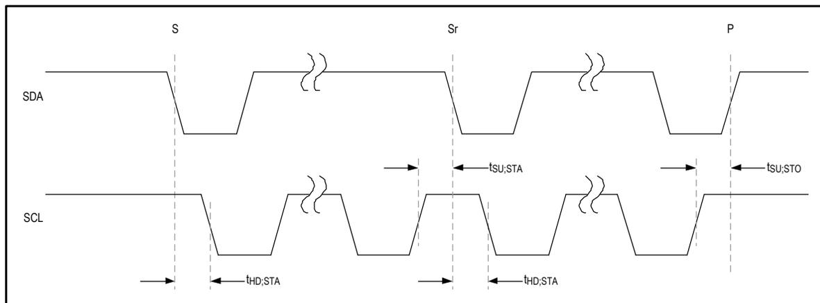
Figure 3. I<sup>2</sup>C START and STOP conditions.
