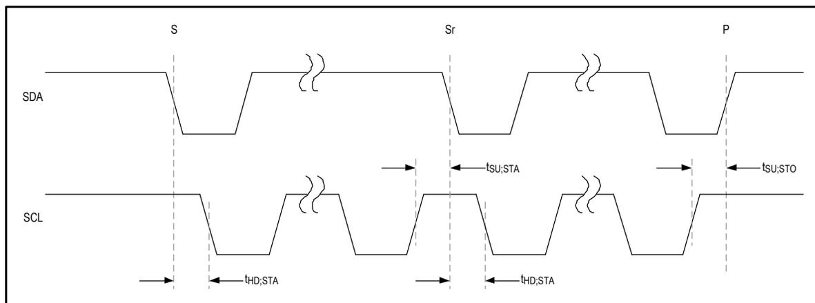
Figure 3. I<sup>2</sup>C START and STOP conditions.
