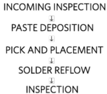
*Figure 3. Recommended uSLIC assembly process.*
