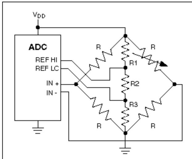
*Ratiometric measurement using resistive bridge network.*
