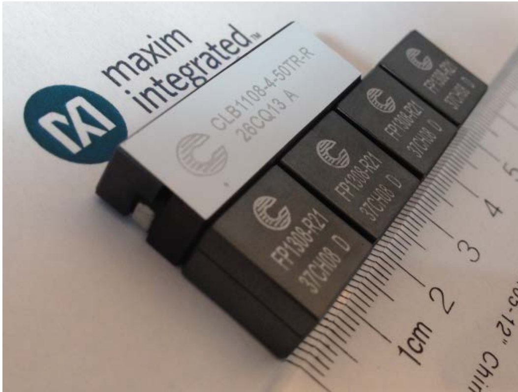
Figure 6. Multiphase coupled inductor CLB1108-4-50TR-R for high-current applications, with large discrete inductors it replaces, 11 .
