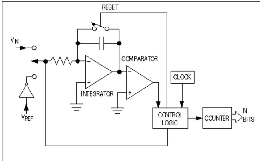
Figure 3. For slowly changing signals, one of the slowest but simplest conversion techniques employs an integrator that charges with the input voltage and discharges with an opposite-polarity reference voltage.
