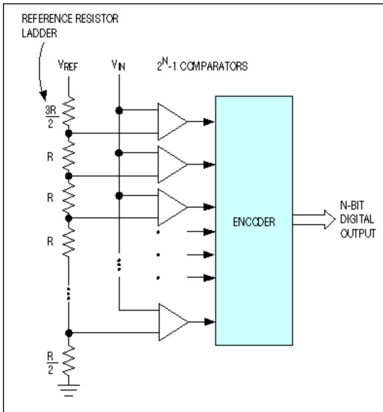
Figure 1. ADCs based on the direct-conversion architecture (better known as flash converters) include  $2^N-1$  comparator banks and a reference resistor-divider network.
