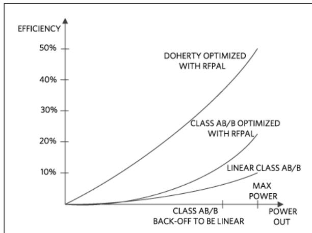
Figure 1. Ideal power-efficiency curves for Class AB/B and Doherty power amplifiers.
