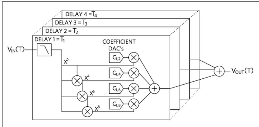
Figure 4. Volterra series block diagram.
