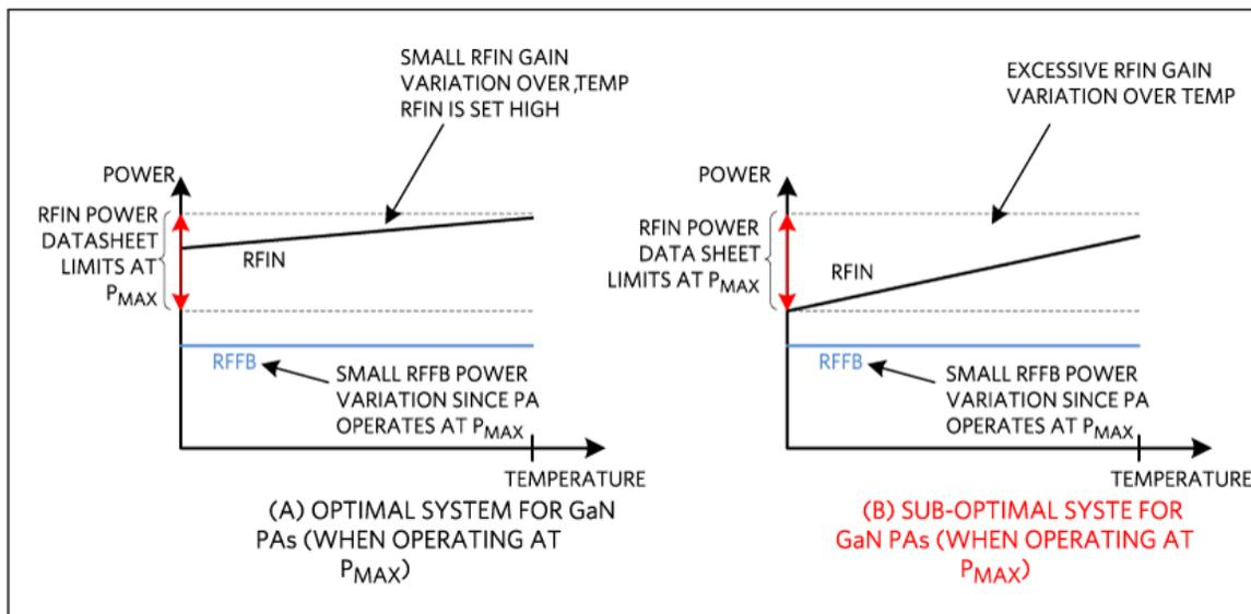
Figure 10. RFIN-range and PA-gain temperature variation.
