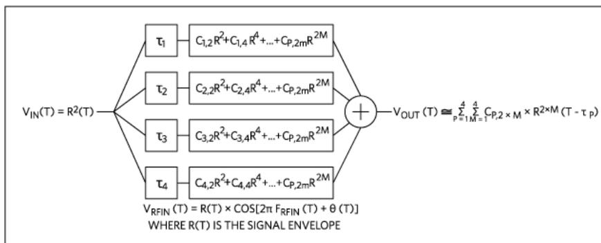
Figure 3. Volterra Series equation.
