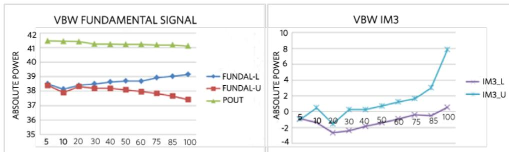
Figure 7. Example VBW measurements on LDMOS Doherty PA.
