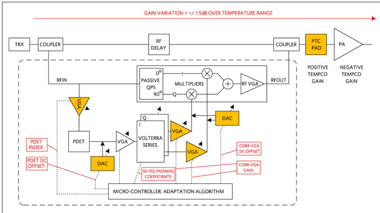
Figure 8. SC1894 correction path block diagram.
