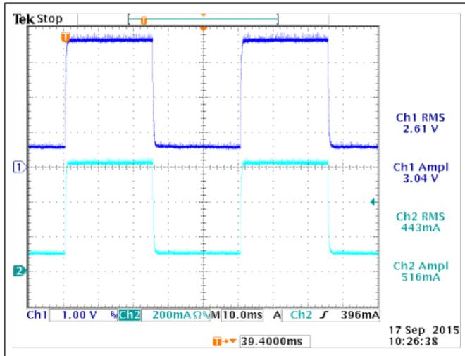
Figure 5. 100mA DC and 600mA transient current loading at 20Hz, 50% duty cycle.
