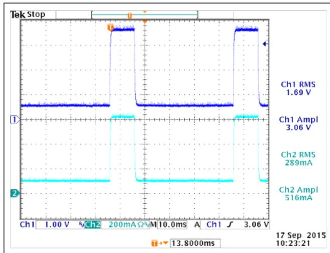
Figure 4. 100mA DC and 600mA transient current loading at 20Hz, 20% duty cycle.
