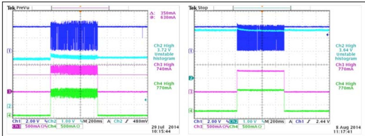
Figure 2. Oscillation with 1x 10 $\mu$ F output capacitor vs. stable operation and vs. unstable operation.
