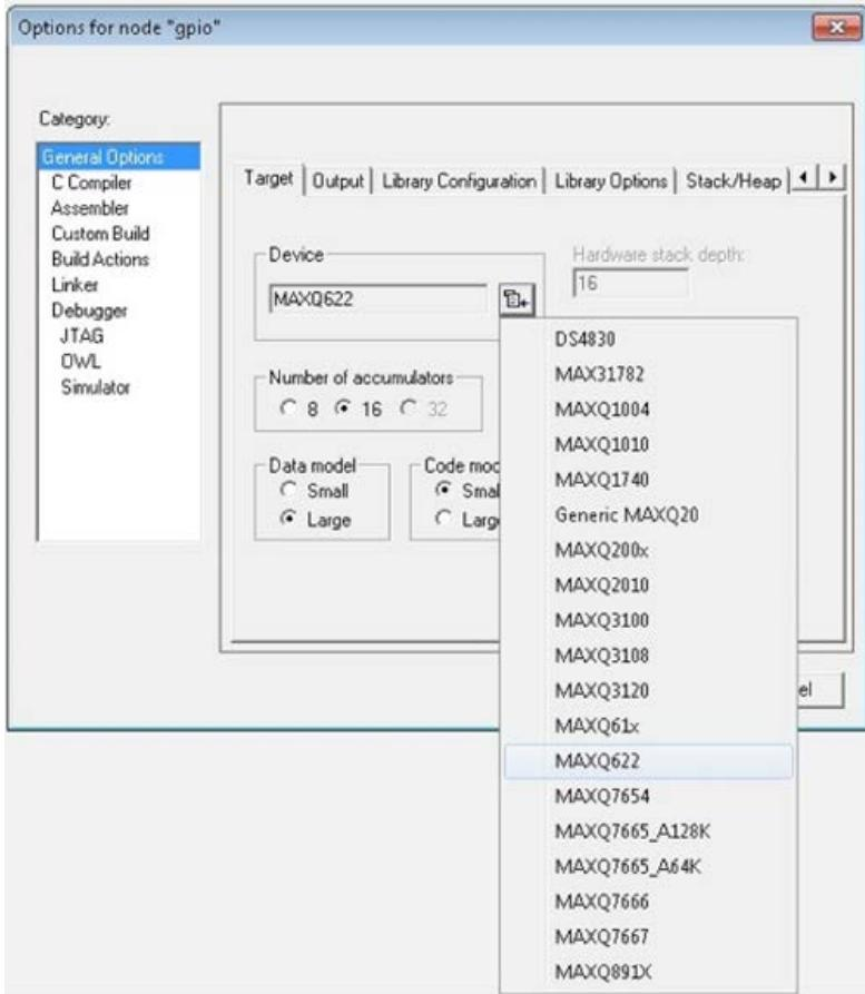
Figure 3. IAR Embedded Workbench project configuration.
