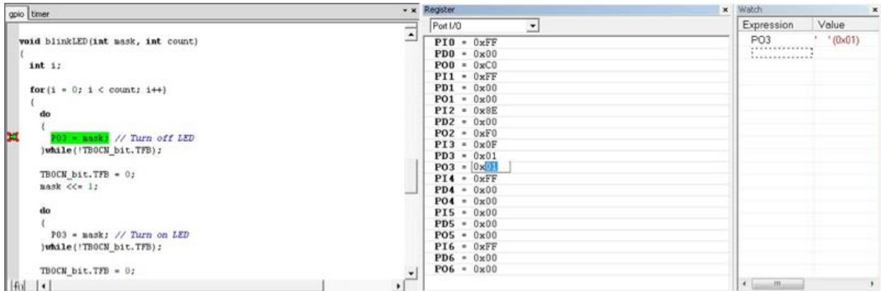
Figure 8. blinkLED() function/IAR Register and Watch.
