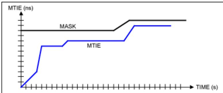
Figure 6. Typical MTIE graph with an MTIE mask.
