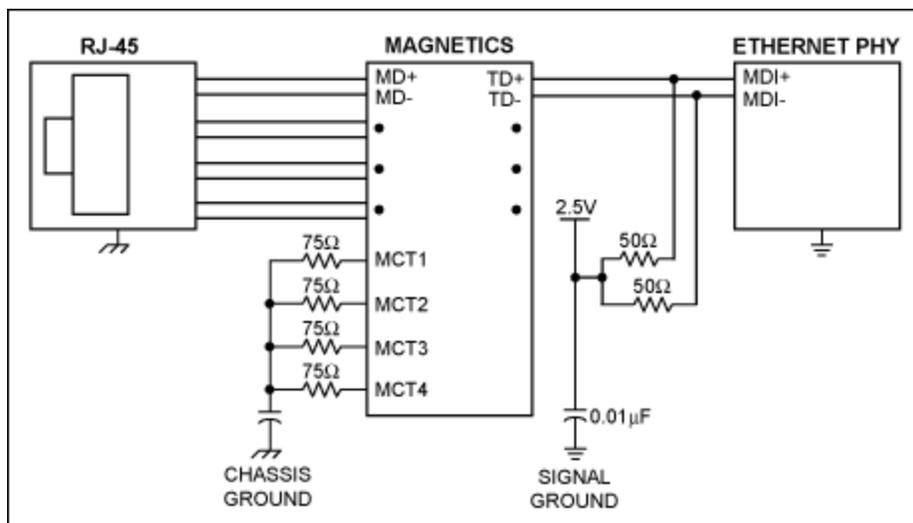
Figure 3. Typical Ethernet PHY connection.
