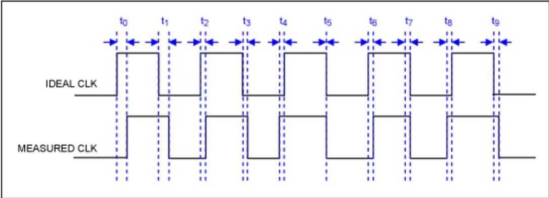
Figure 4. TIE measurement against an ideal source.
