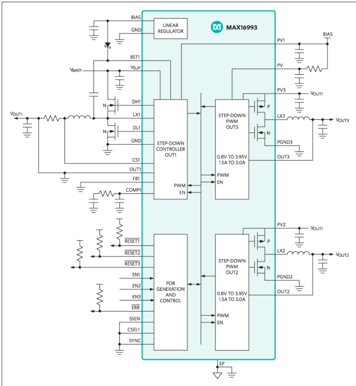
Figure 4. The Maxim MAX16993 DC-DC step-down power controller provides one higher-voltage output and two lower-voltage outputs, specifically optimized in performance and capability for automotive situations.
