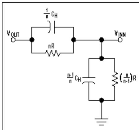
Figure 6. Equivalent circuit of feedback network.
