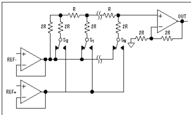
Figure 1. Simplified DAC circuit.
