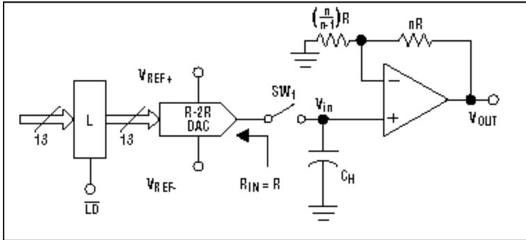
Figure 3. An improved deglitch circuit.
