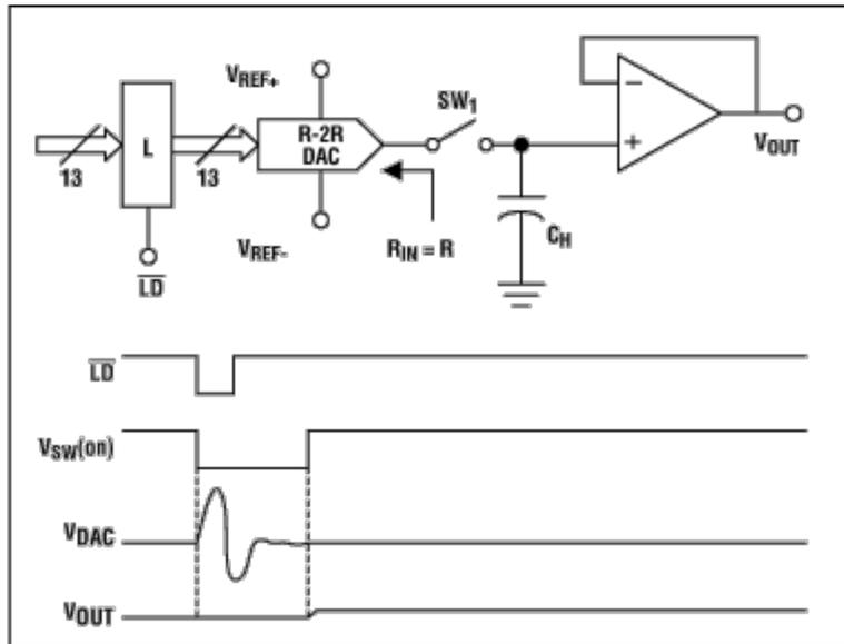
Figure 2. Integrated T/H deglitch architecture.
