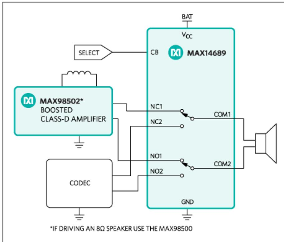
Figure 1. Solution for typical audio setup.
