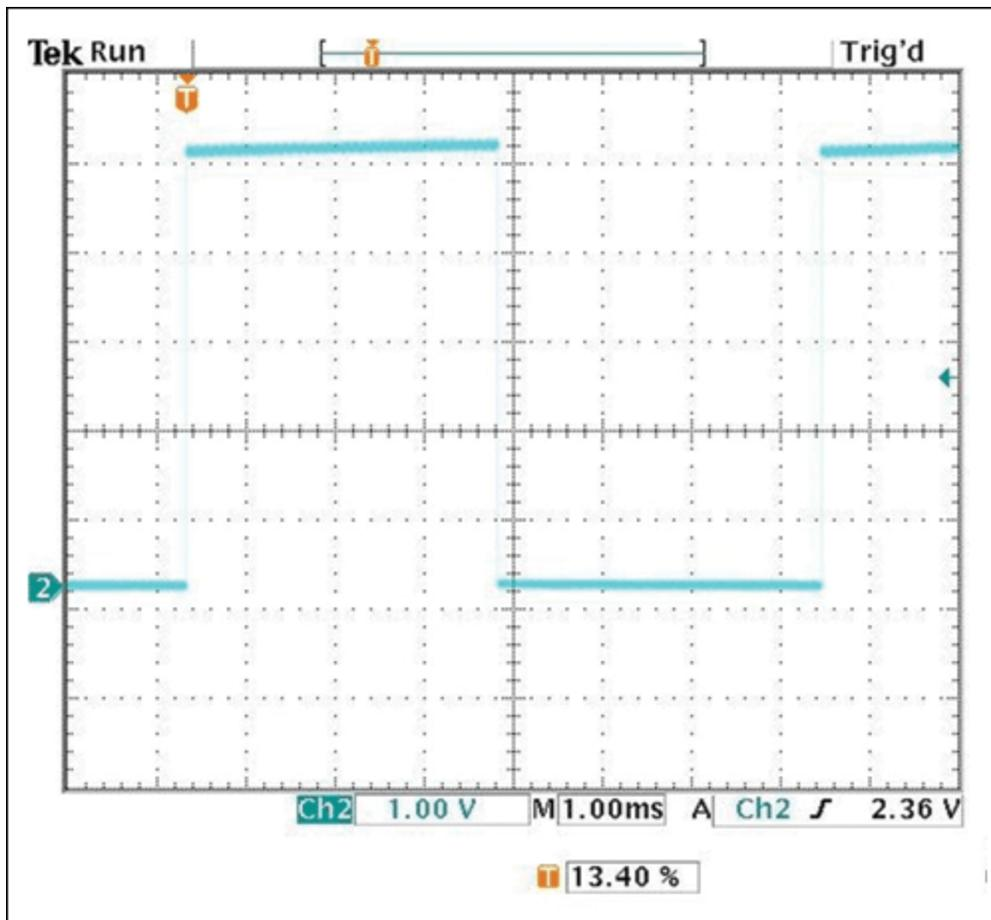
Figure 4. PWM output with no control voltage.
