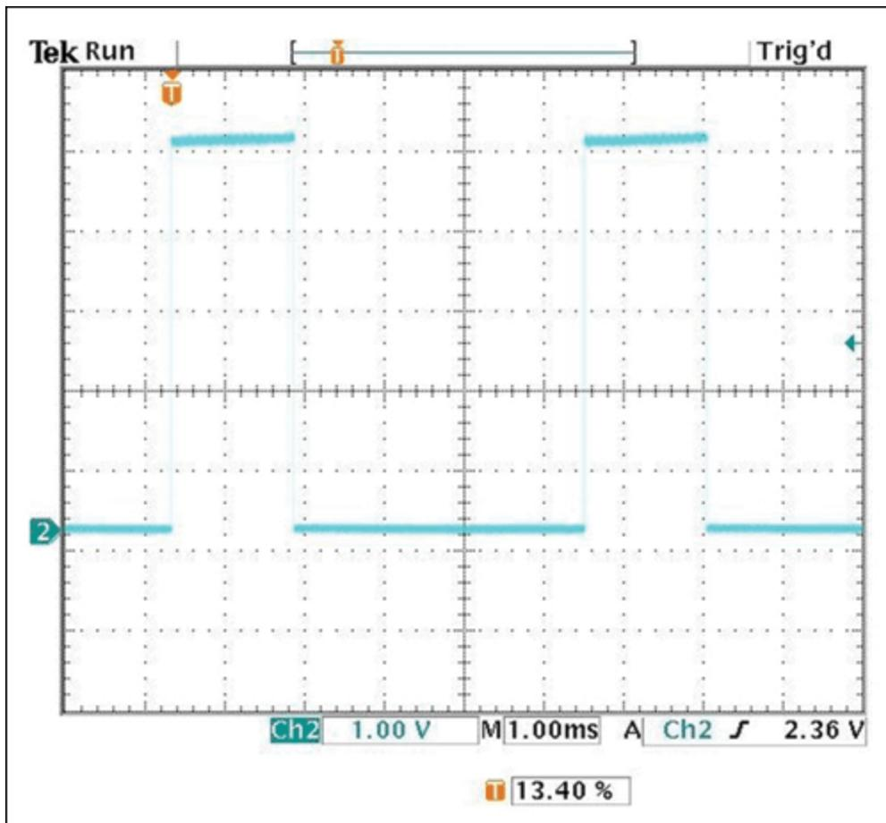
Figure 3. PWM output with control voltage = 2V.
