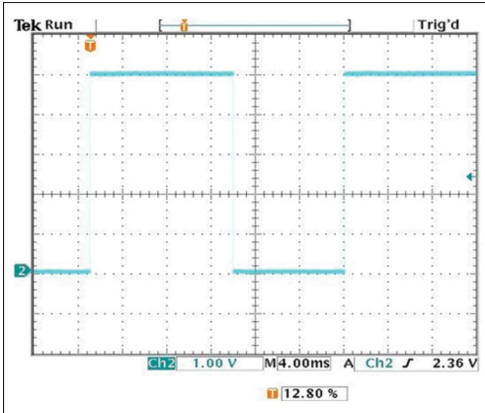
Figure 9. PWM output with control voltage = 3V.
