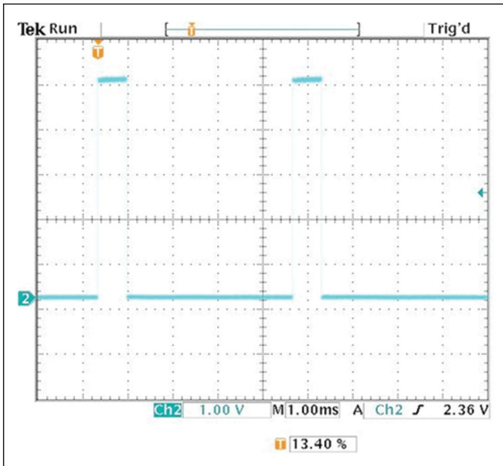
Figure 2. PWM output with control voltage = 1V.
