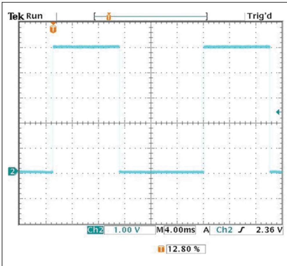
Figure 8. PWM output with control voltage = 2V.
