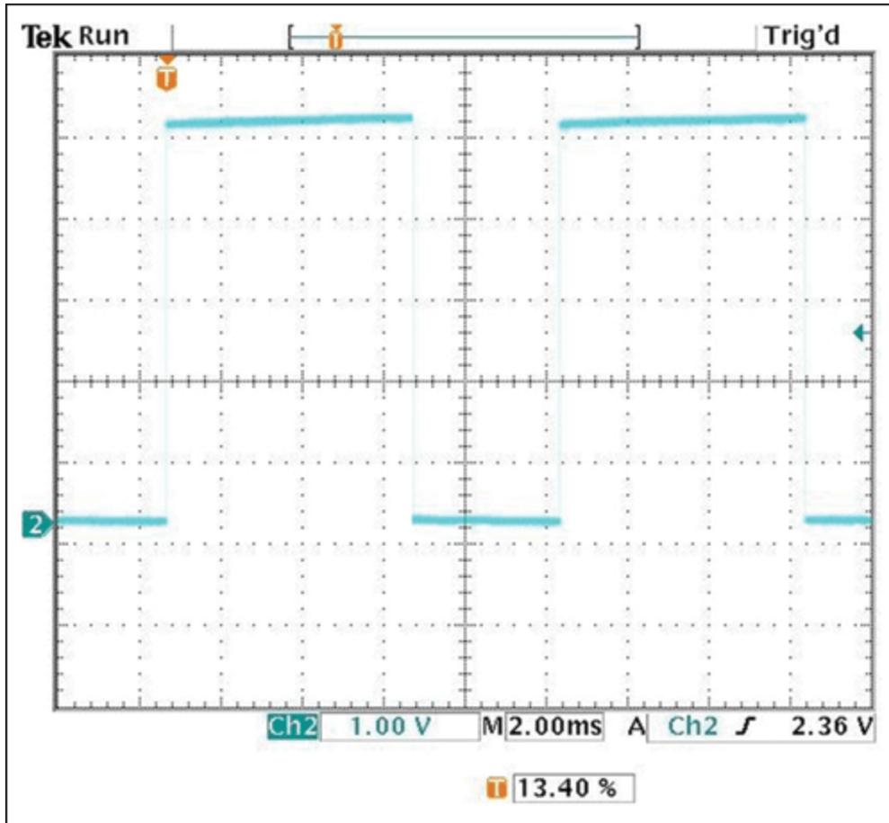
Figure 5. PWM output with control voltage = 4V.
