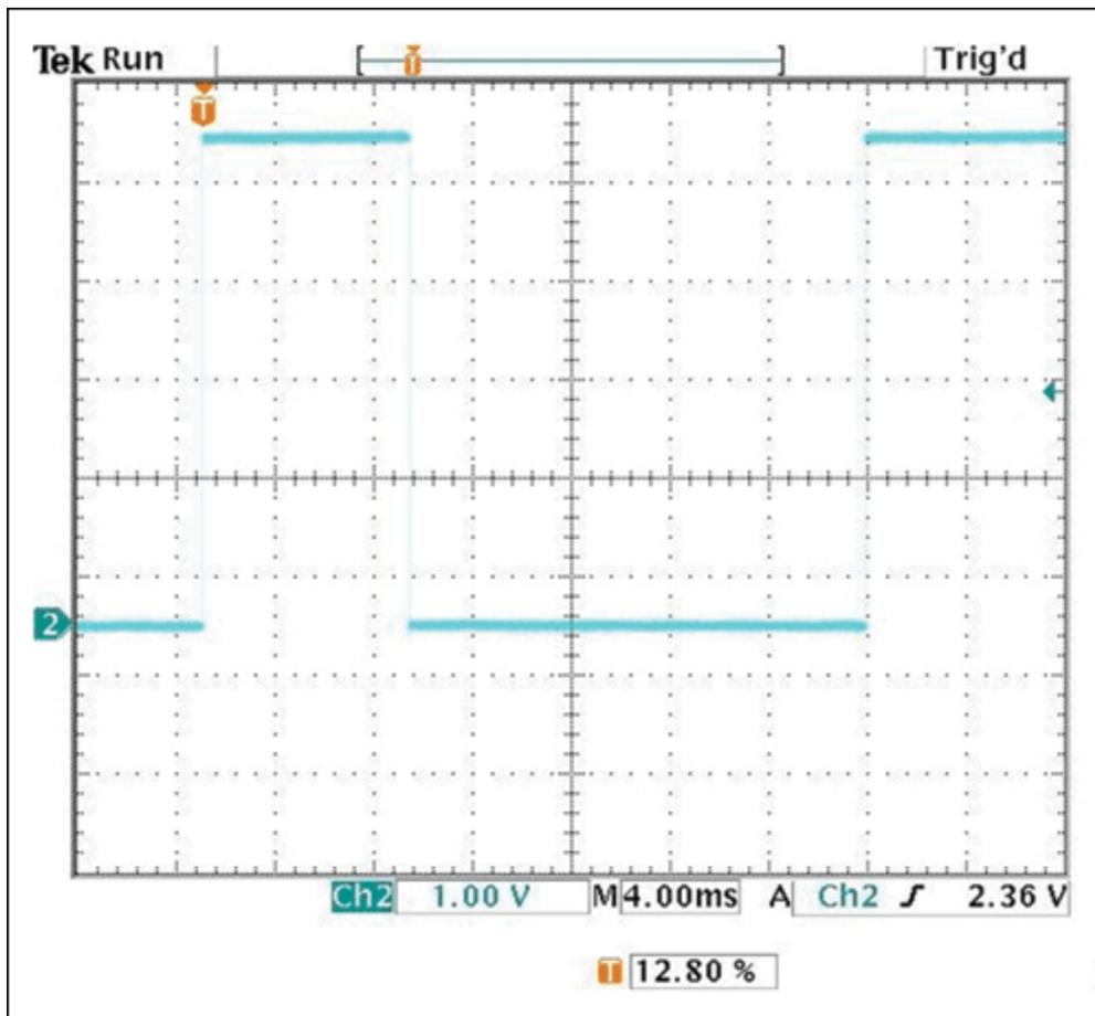
Figure 7. PWM output with control voltage = 1V.
