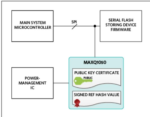
Figure 2. A typical block diagram with the MAXQ1050 secure microcontroller used as a secure coprocessor.
