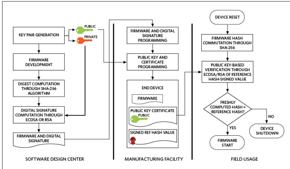
Figure 1. A secure boot flow across device life-cycle phases.
