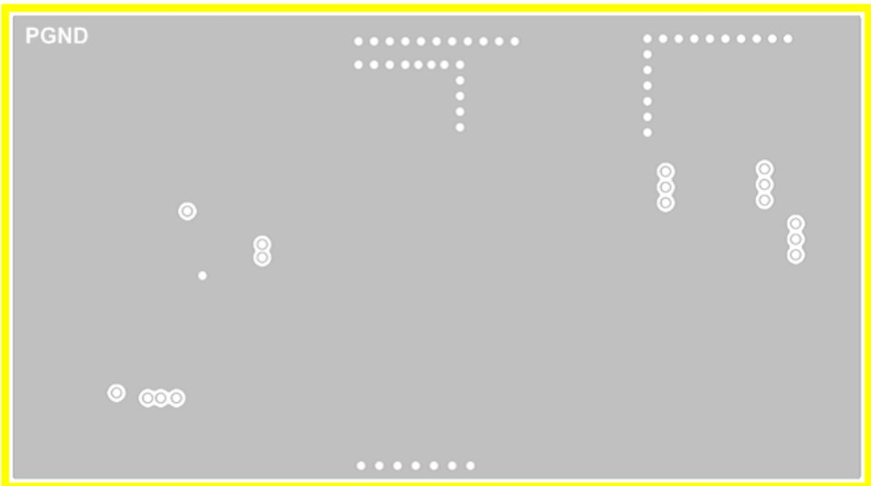
Figure 9. Reference design layout, inner layer 1.
