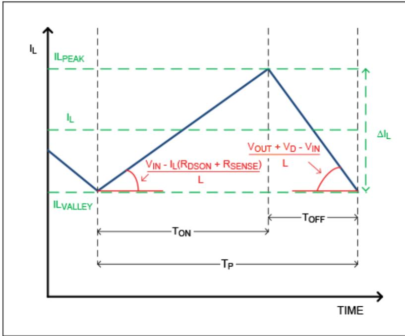
Figure 1. Inductor current of the boost regulator.
