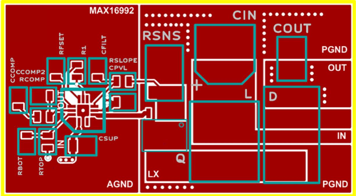
Figure 8. Reference design layout, top layer.
