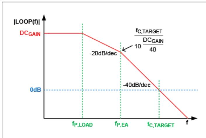
Figure 3. Bode diagram of the amplitude of the closed-loop response, case 1.
