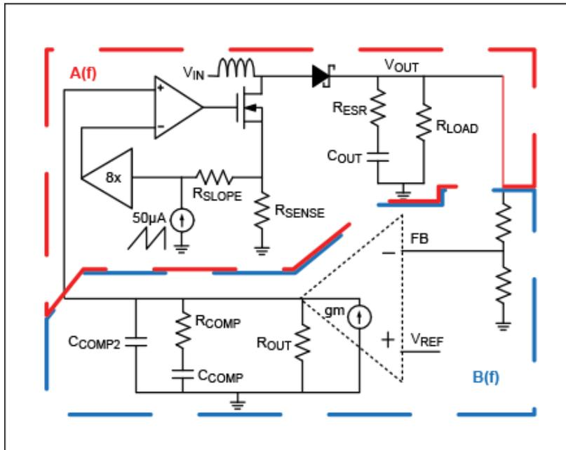
Figure 2. Boost regulator small-signal model.
