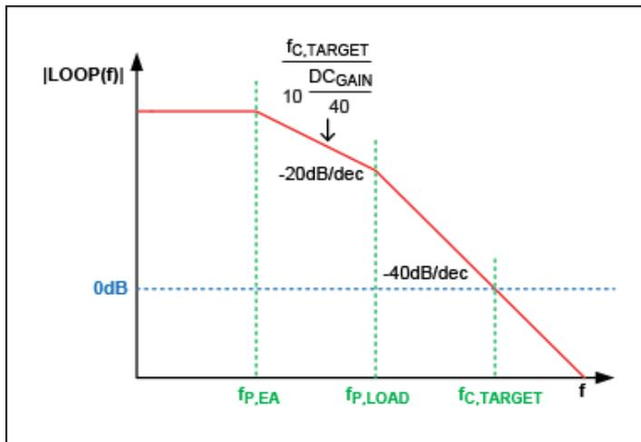
Figure 4. Bode diagram of the amplitude of the closed-loop response, case 2.
