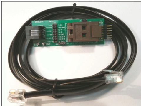
Figure 1. The DS9120P EV board with RJ11 cable.
