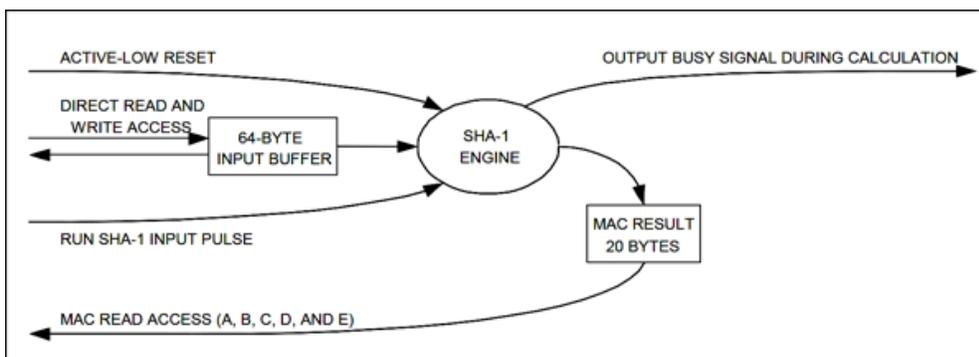
Figure 2. Data flow diagram.
