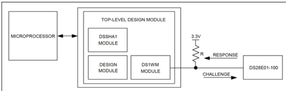
Figure 5. Typical FPGA or ASIC application.
