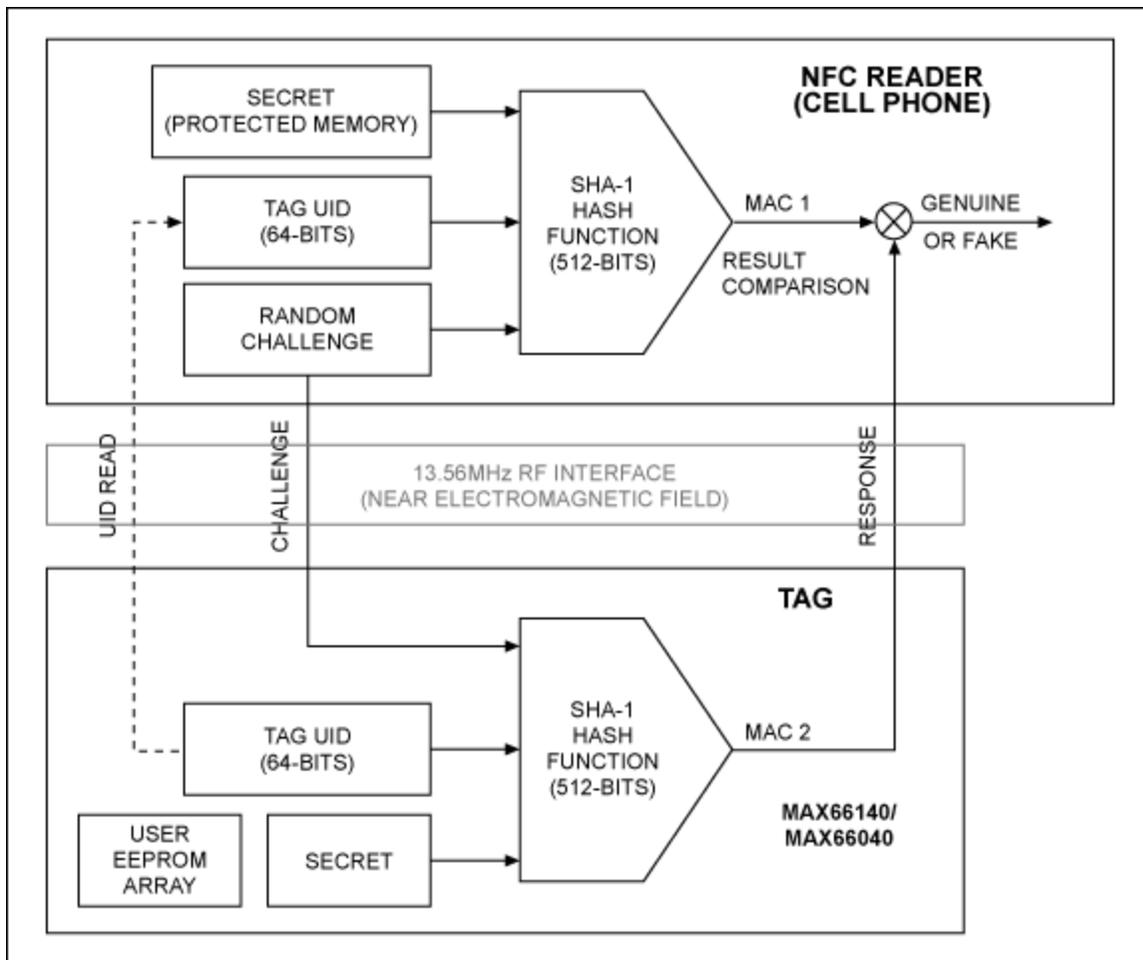
Figure 1. SHA-1-based challenge-response authentication principle.
