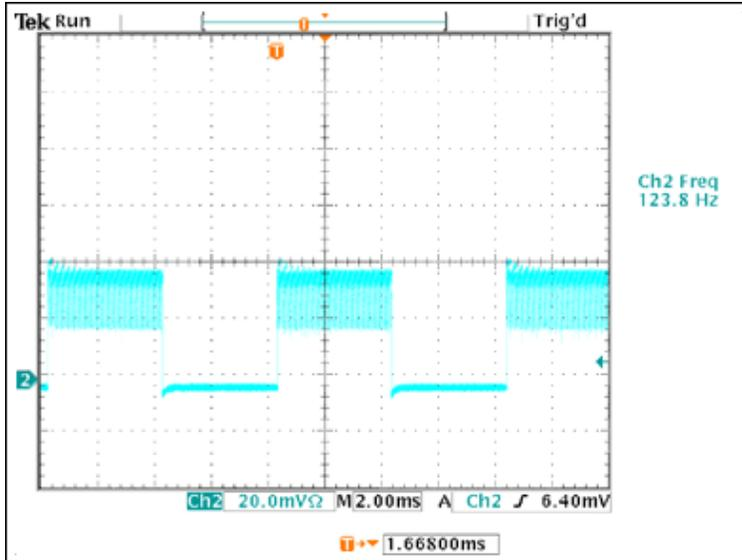
Figure 3b. LED current with an 85% external PWM duty cycle.
