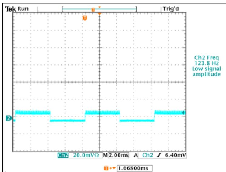
Figure 3a. LED current with a 15% external PWM duty cycle.
