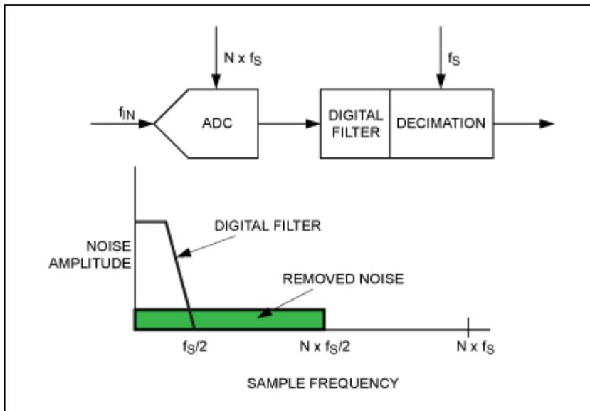
Figure 2. ADC with oversampling by a factor of  $N$ , digital filter, and decimation.
