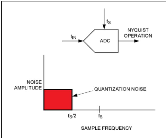
Figure 1. Standard ADC noise performance.
