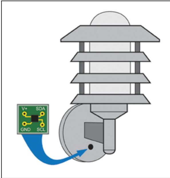
*Figure 1. The ALS is mounted on a separate PCB and placed underneath the shadow of the luminaire's support beam. This prevents the sensor from reading light from the lamp itself.*
