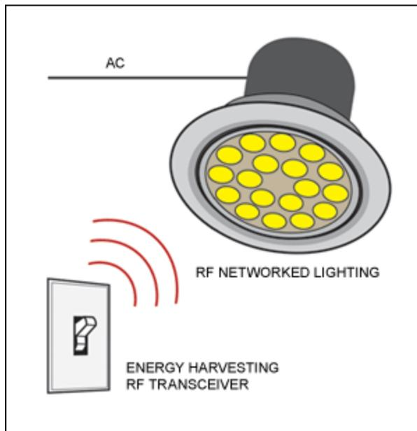
*Figure 2. A building automation application in which the light switch contains an unwired, energy-harvesting RF transceiver that controls the LED lighting.*
