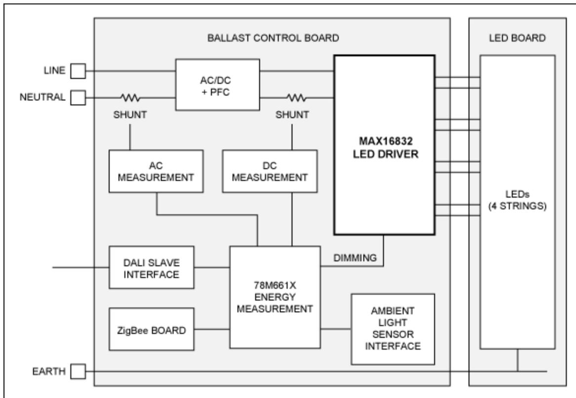
Figure 4. A complete smart LED lighting reference design, featuring energy measurement, ambient light sensing, and communication.
