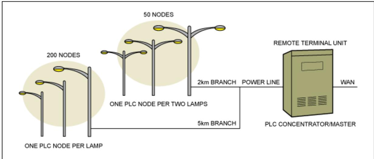
Figure 3. An example of a municipal streetlight network using PLC.<sup>4</sup>
