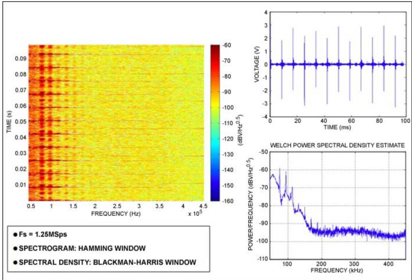
Figure 1. Channel noise on LV line. Image courtesy of Texas Instruments.
