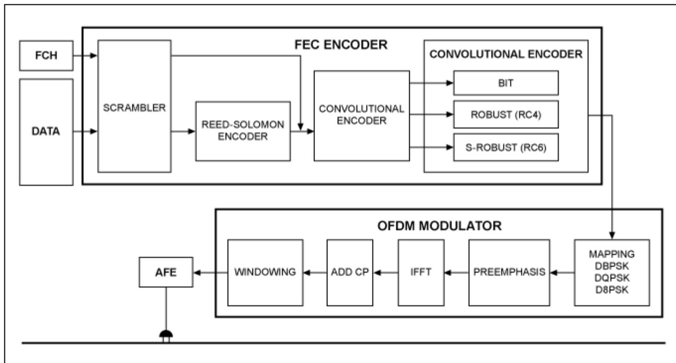
Figure 4. Forward error correction block diagram.
