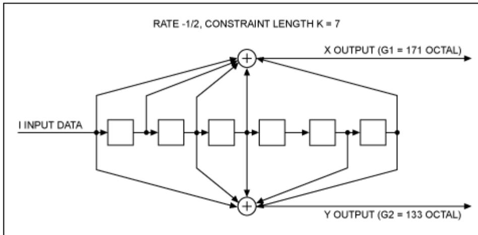
Figure 6. Convolutional encoder.
