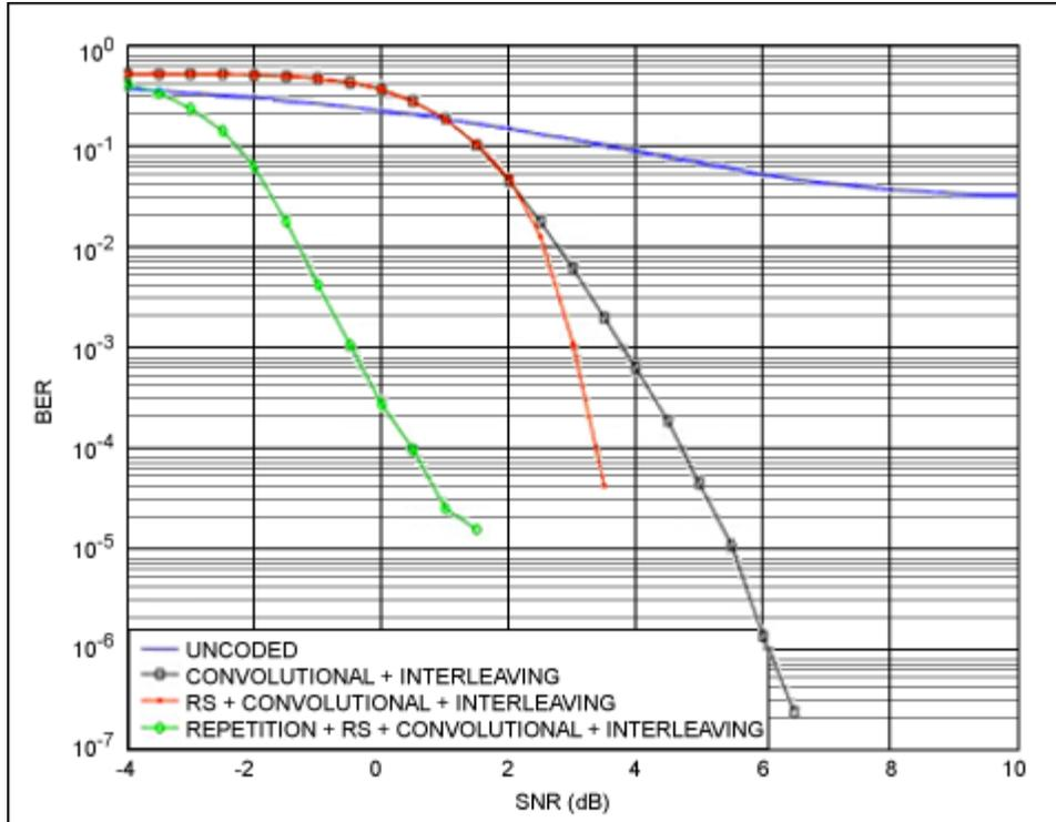
Figure 7. Simulated BER versus SNR performance improvements with added error correction.
