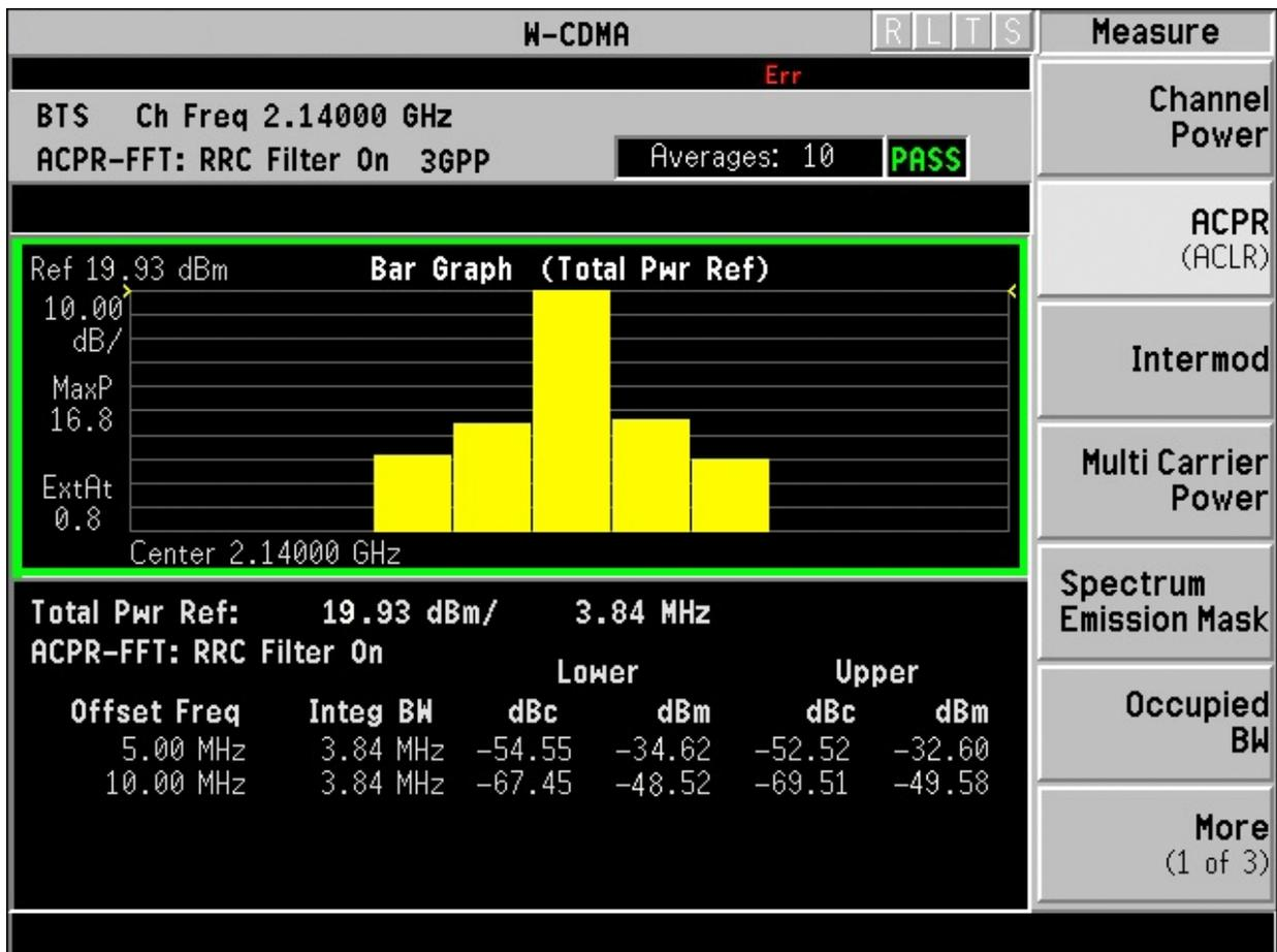
Figure 4. TM1 16DPCH signal ACLR at +20dBm output power level.
