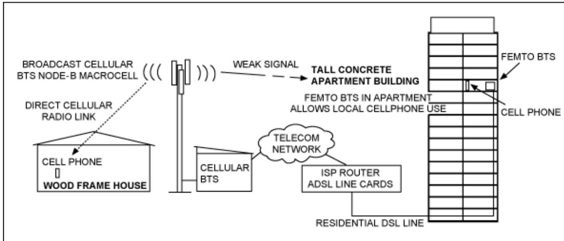
Figure 1. Traditional node-B macrocell cellular connection vs. femtocell base station connection.
