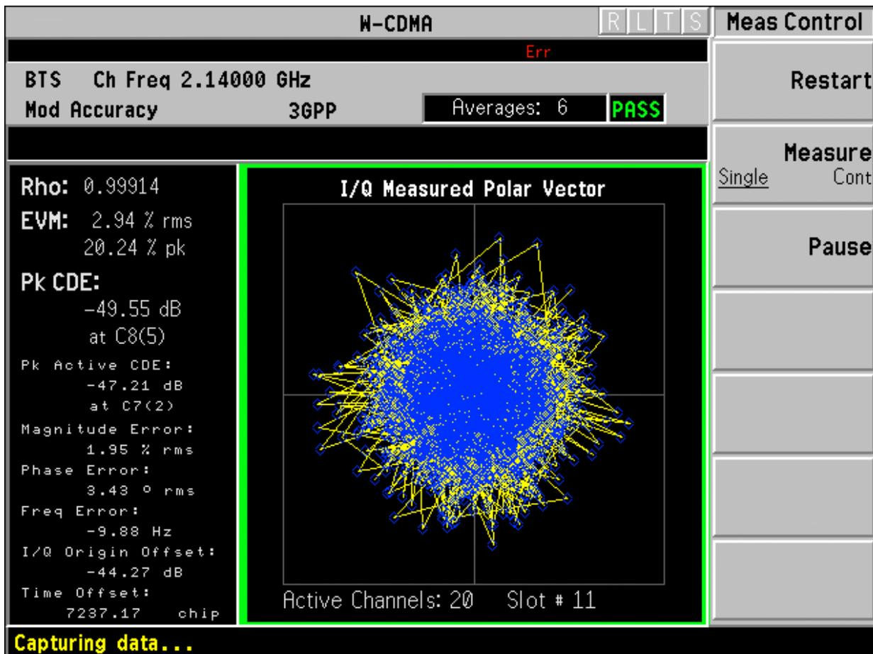
Figure 5. TM1 16DPCH signal EVM at +20dBm output power level.
