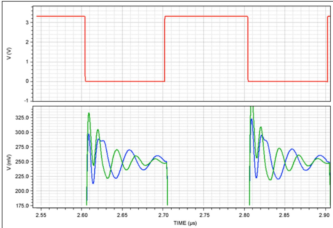
Figure 9. Switched capacitor voltage with ferrite bead at ADC input.
