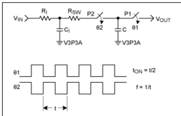
Figure 3. Switched capacitor network with RC Input.
