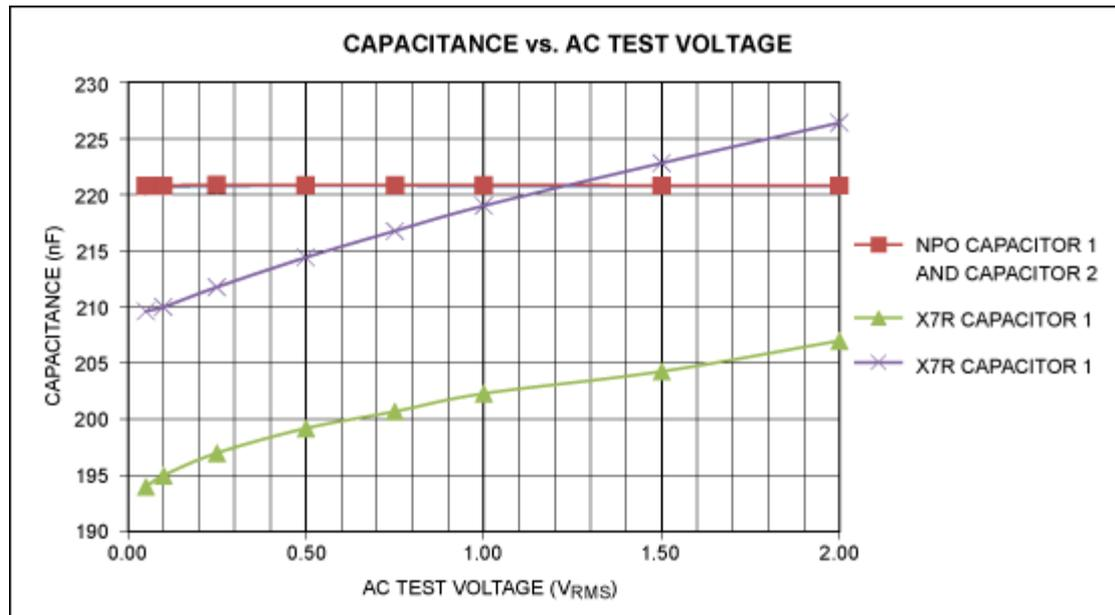
Figure 4. The effect of a 50Hz amplitude signal on NPO-type and X7R-type capacitors.
