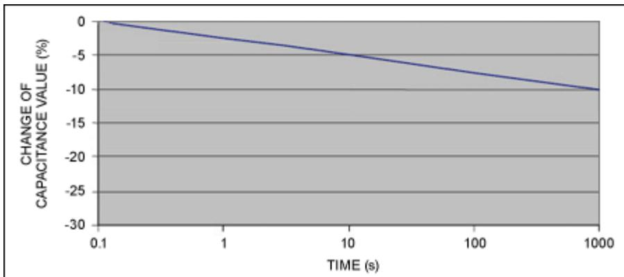
Figure 6. The effects of aging capacitors.
