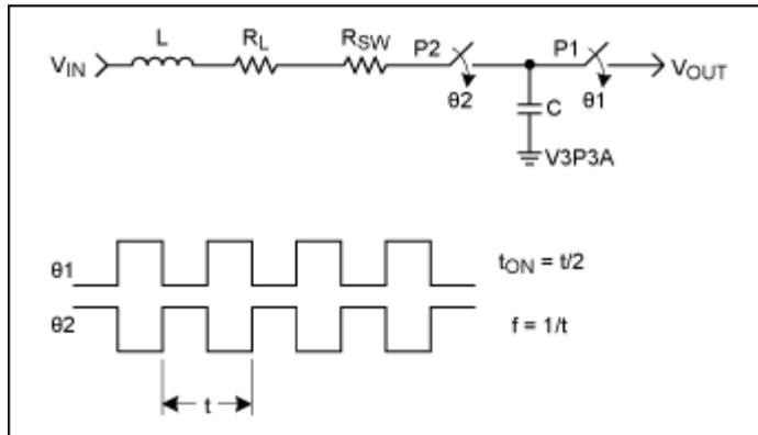
Figure 7. Simplified equivalent circuit of the switched capacitor network with ferrite bead.
