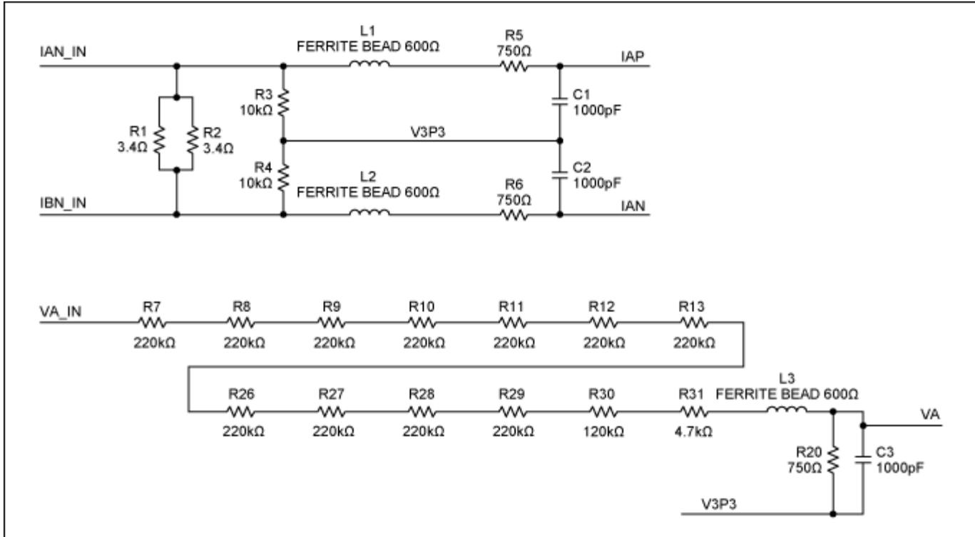
Figure 10. Recommended ferrite bead placement near ADC input.
