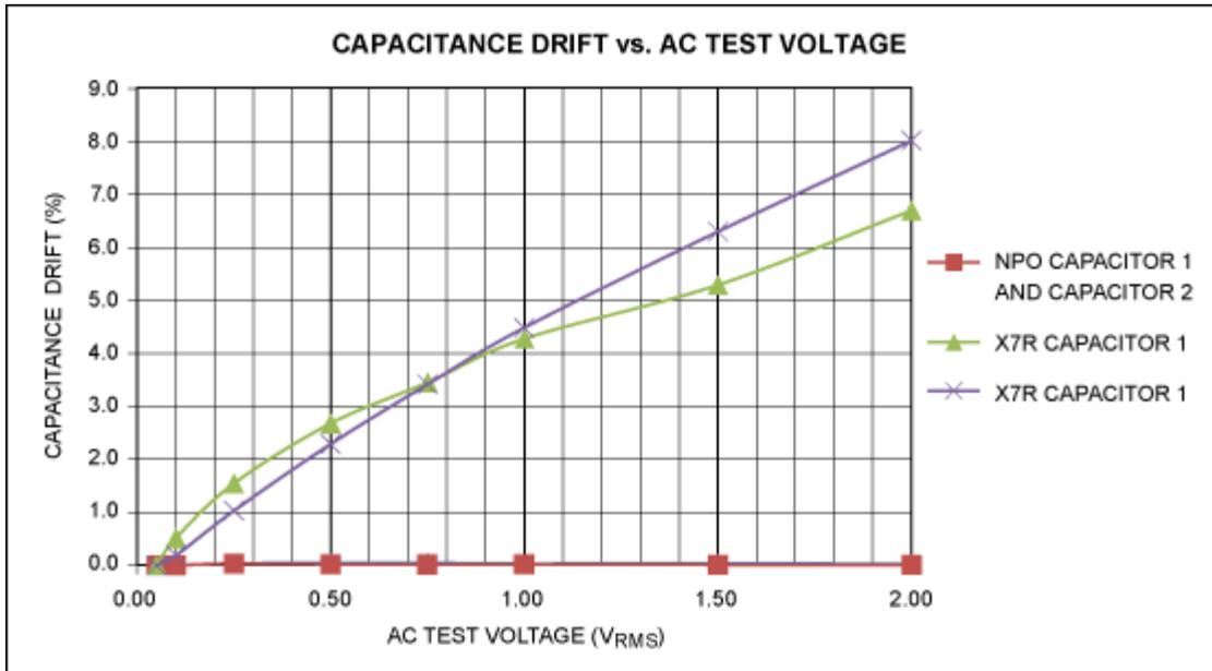
Figure 5. Inaccuracy due to capacitance drift.
