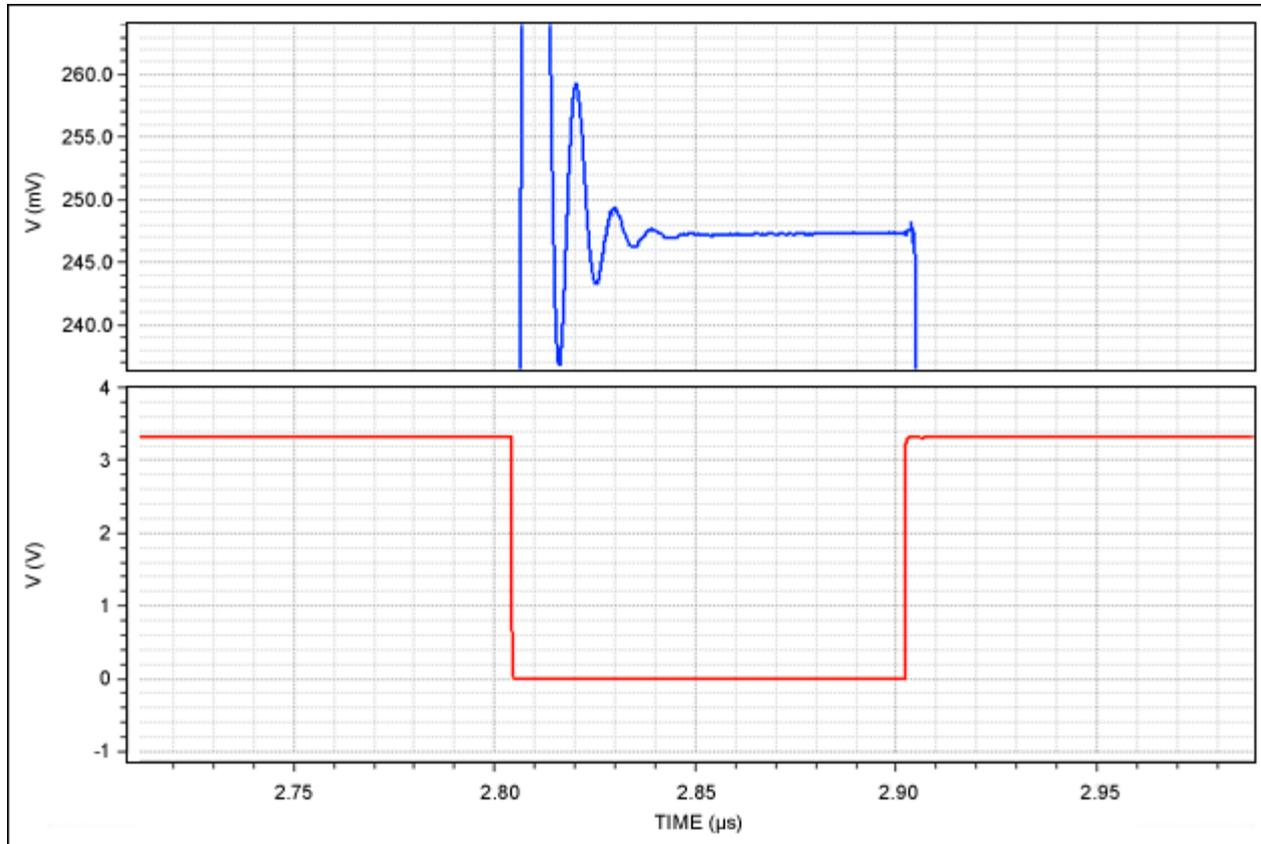
Figure 11. Switched capacitor voltage with ferrite bead and RC at ADC input.
