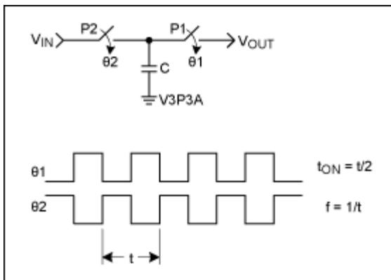
Figure 1. Simplified equivalent circuit of a switched capacitor input network.
