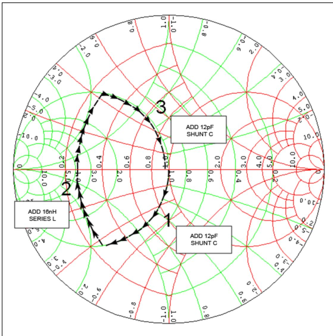
Figure A1. Impedance/admittance contours for a 50Ω pi filter at 433.92MHz.
