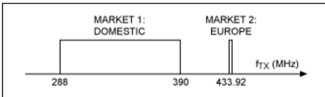
Figure 2. Relative positions of domestic and European low-band frequencies.
