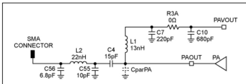
Figure 3. Diagram of the MAX7060 match and filter for improved efficiency at +10dBm.
