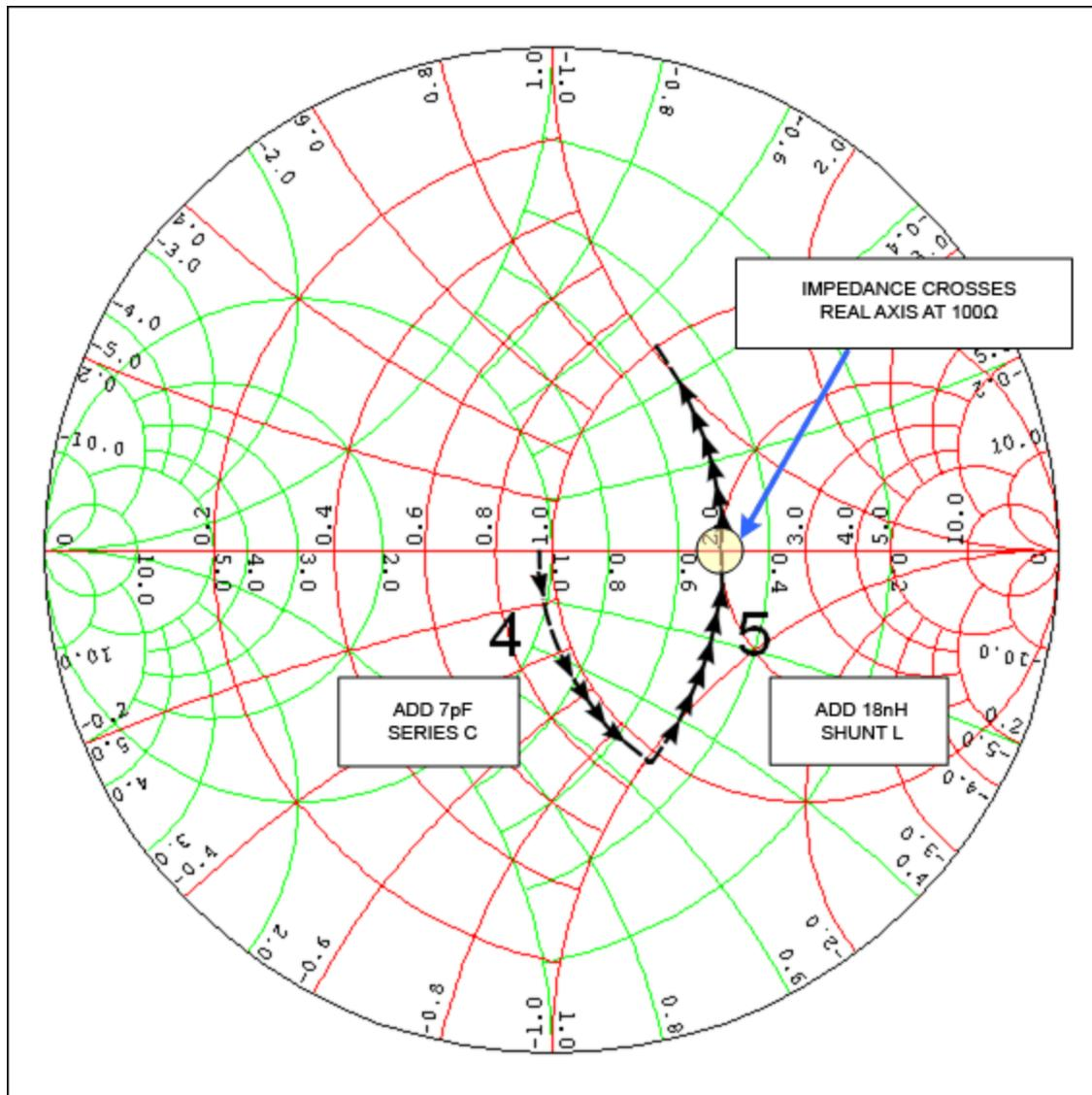
Figure A2. Impedance/admittance contours for a  $50\Omega$  to  $100\Omega$  transformation at  $433.92\text{MHz}$ .
