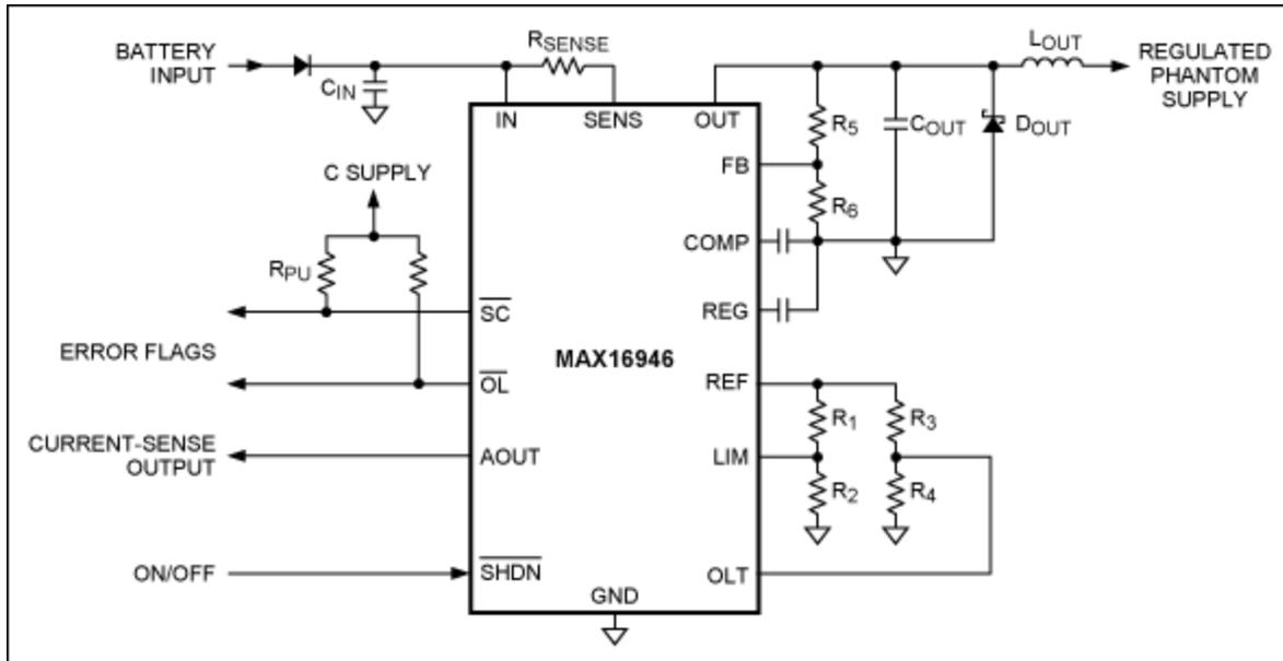
Figure 1. Typical operating circuit of the MAX16946 remote antenna CSA and switch.
