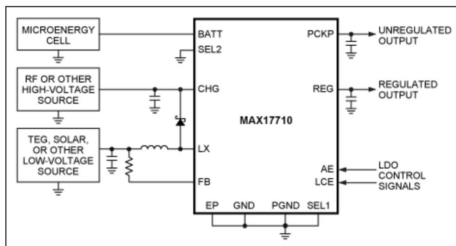
Figure 2. The MAX17710 shown in a typical application circuit harvesting from high-voltage charge sources.
