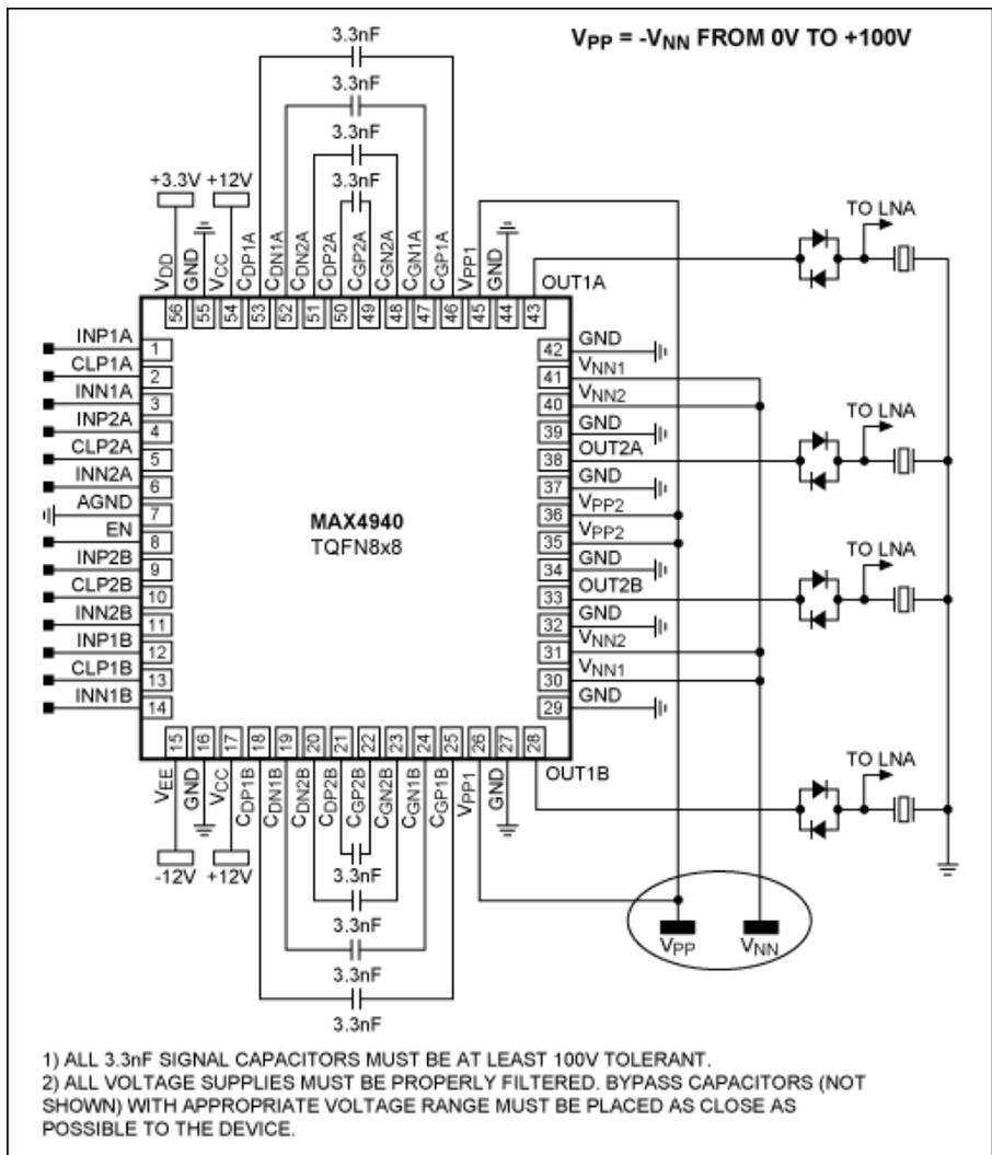
Figure 3. Typical application circuit of the MAX4940 quad, bipolar digital pulser.
