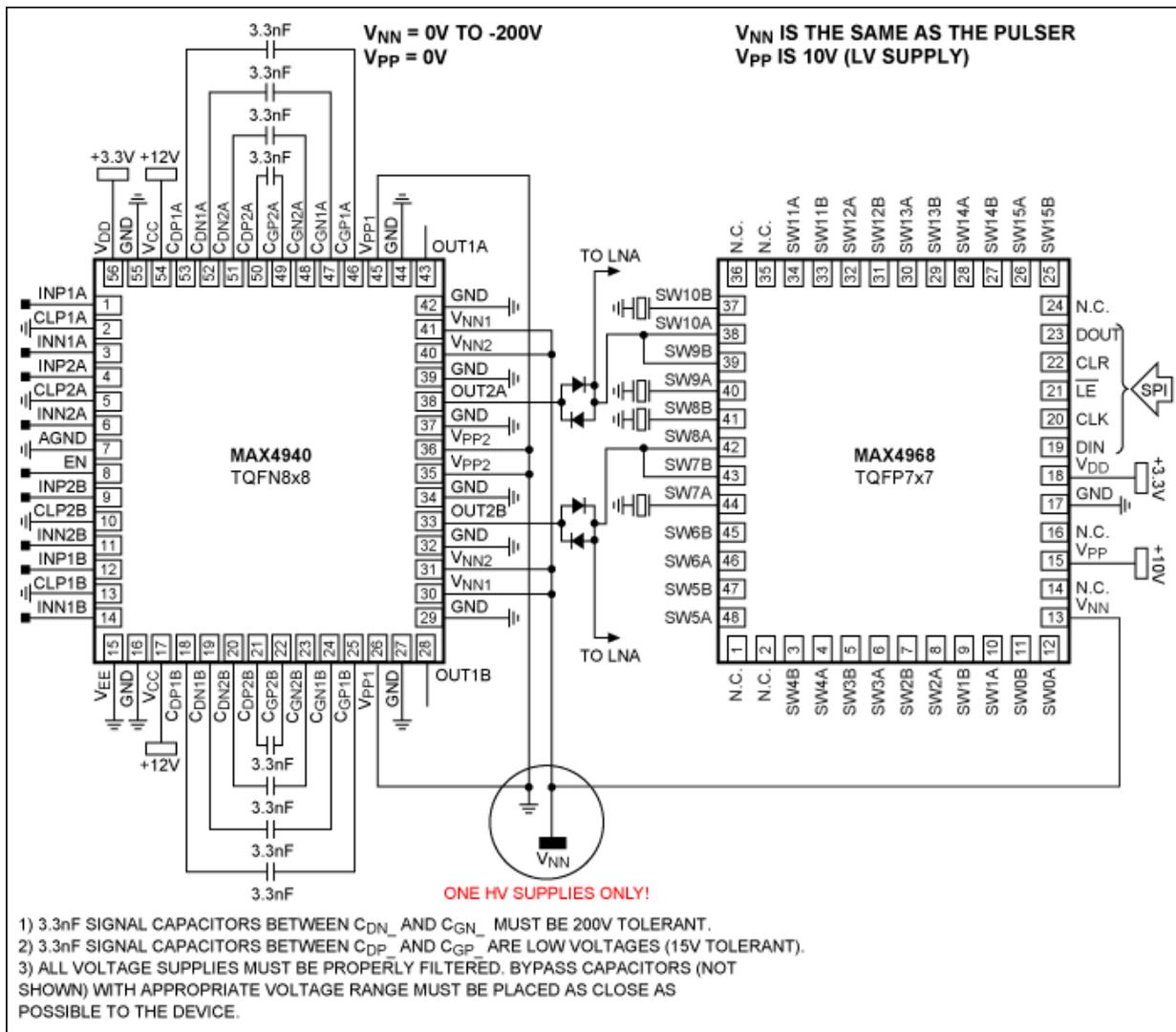
Figure 10. Use of MAX4968 and MAX4940 together in unipolar negative applications reduces the number of HV supplies needed.
