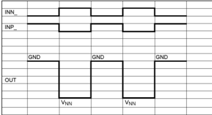
Figure 11. Signal timing diagram for pulsing and switching using MAX4940 and MAX4968 in unipolar negative applications.
