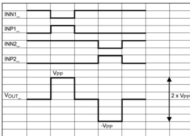
Figure 13. Timing diagram of a typical driving scheme in BTL configuration.
