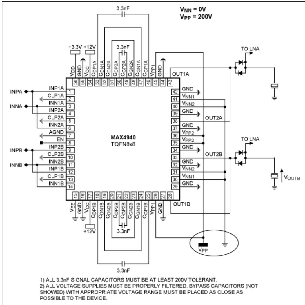
Figure 14. Application diagram of a 4A positive unipolar pulser.
