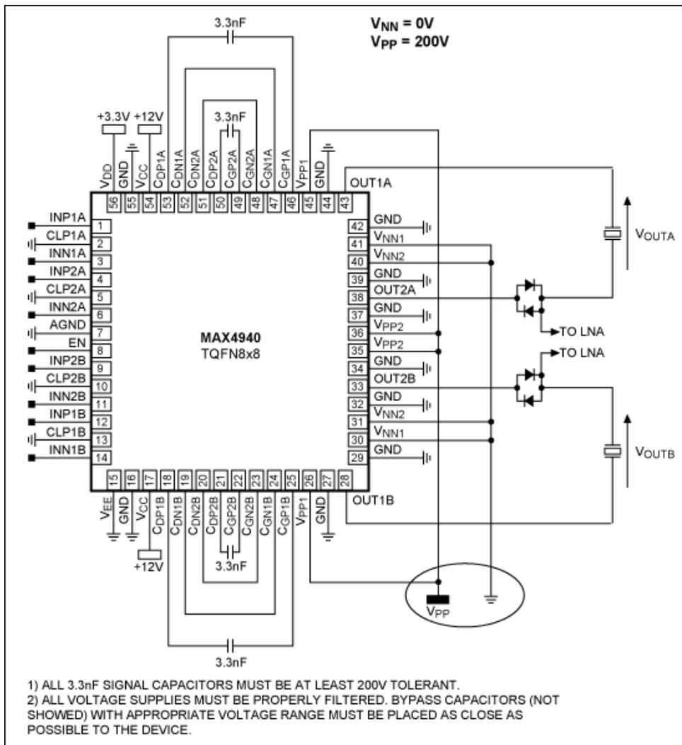
Figure 12. A typical bridge-tied load (BTL) configuration using the MAX490.
