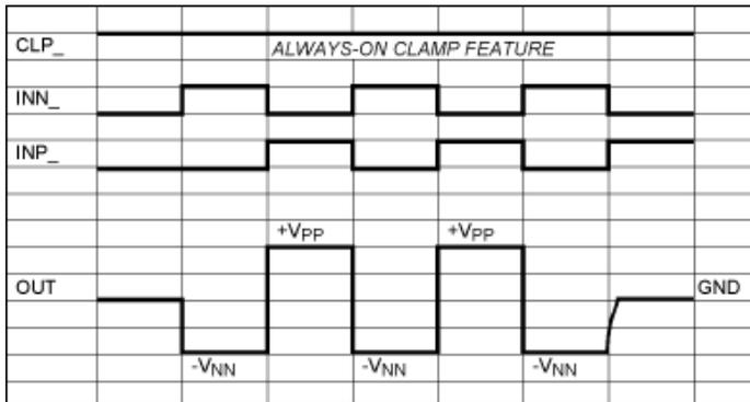
Figure 5. Signal timing diagram for pulsing and switching using the MAX4940 and MAX4968 in bipolar negative applications.
