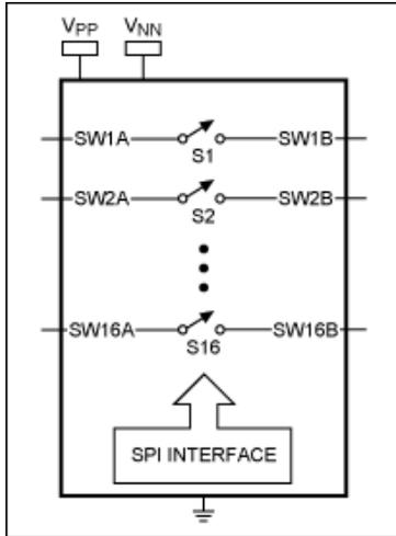
Figure 2. The MAX4968 functional diagram.
