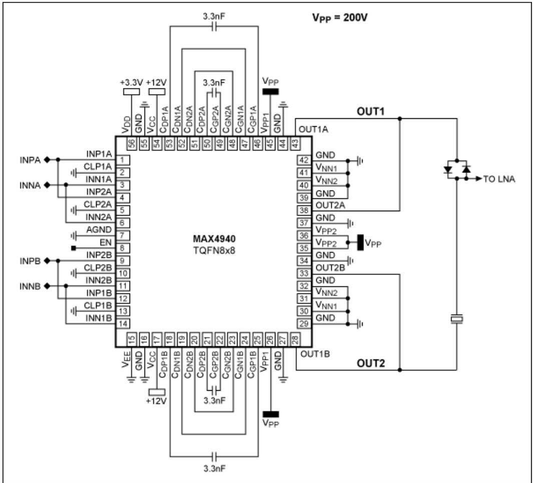
Figure 15. Application diagram of the MAX4940 driving 4A in BTL application.
