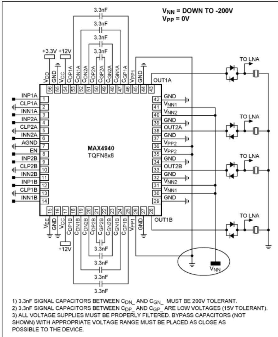
Figure 9. Use of MAX4940 in unipolar applications.
