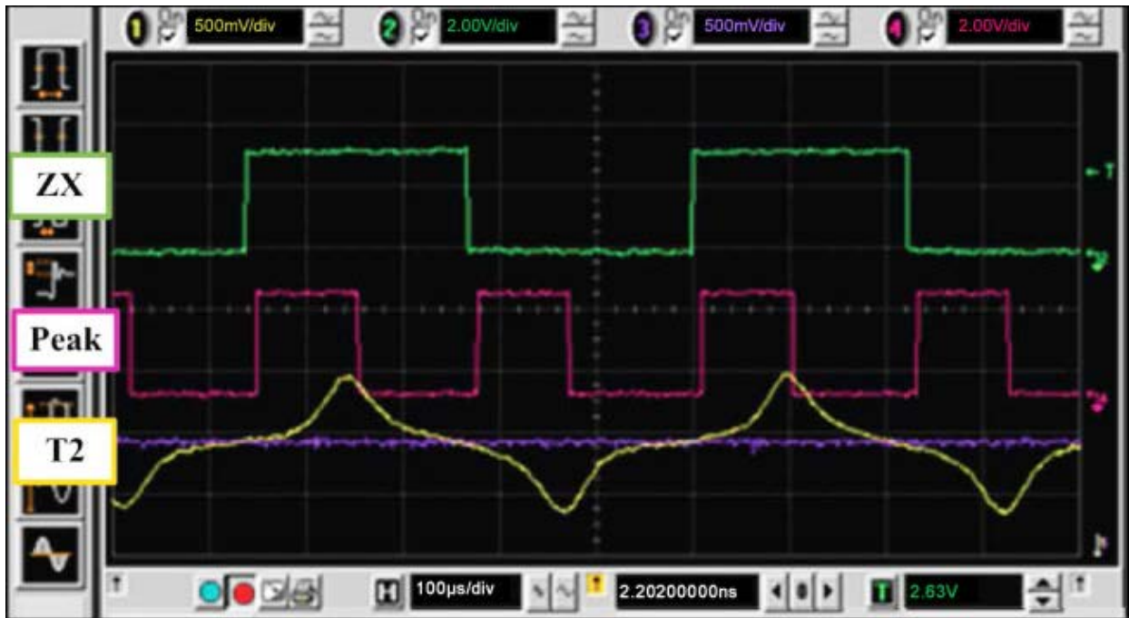
Figure 14. Critically damped behavior. T_2 for a manual swipe with 40% card and R_o = 13.5k\Omega .
