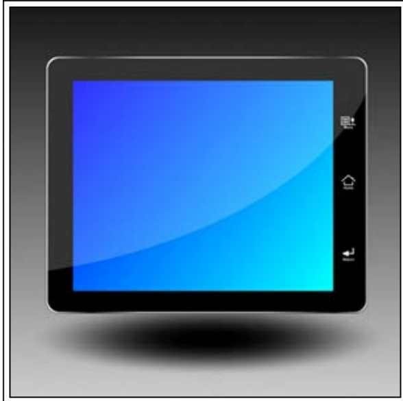
Figure 5. A typical tablet design shows the use of a black border panel around the LCD display. The presence of an ambient light sensor is hidden from the view of the user.
