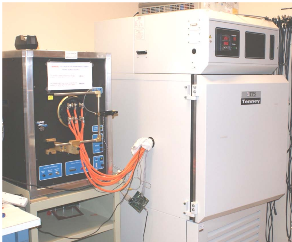
Figure 15: Calibration System with Temperature Chamber
