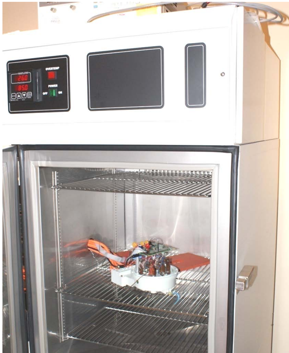
Figure 16: Meter Base with VAC CTs and Demo Board
