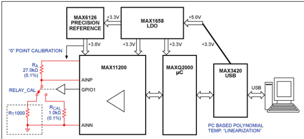
Figure 6. Block diagram of the precision data-acquisition system (DAS) used for measurements in this article. Based on the MAX11200 ADC (Figure 3), the DAS includes a provision for simple calibration and computer-generated linearization.
