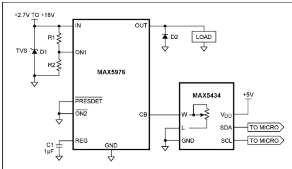
Figure 4. The MAX5976 combined with a nonvolatile digital potentiometer, the MAX5434, for programmable overcurrent limit.
