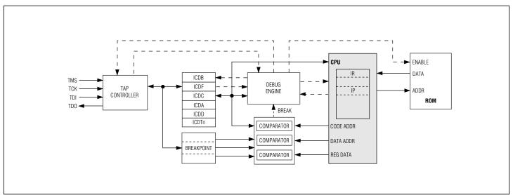
Figure 16-1. In-Circuit Debugger
