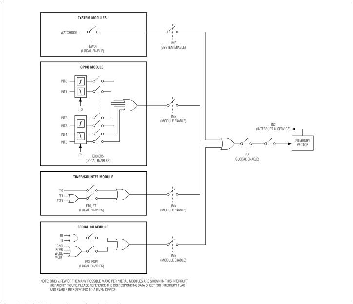
Figure 2-10. MAXQ Interrupt Source Hierarchy Example
