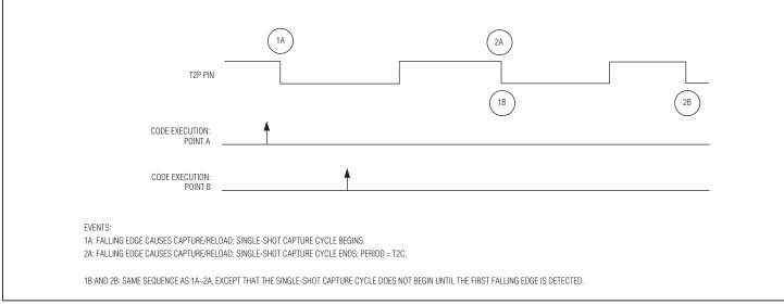
Figure 9-6. Timer 2 Application Example—Measure Period
