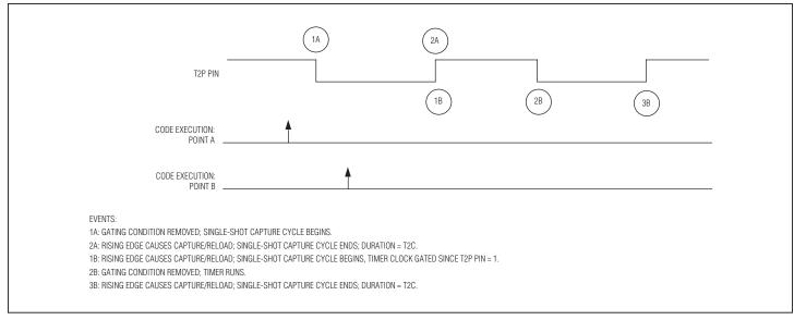
Figure 9-4. Timer 2 Application Example—Measure Low Pulse Width
