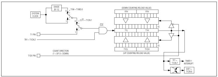
Figure 8-3. Timer/Counter 1 16-Bit Up/Down Count with Auto-Reload
