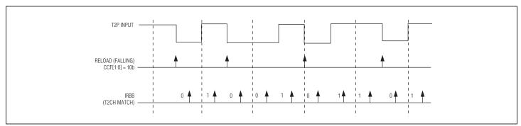
Figure 9-13. Biphase Decoding Example
