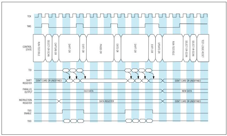
Figure 15-4. TAP Controller Debug Mode DR-Scan Example
