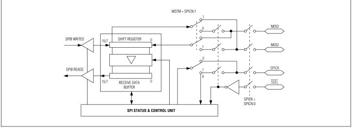
Figure 11-1. SPI Block Diagram
