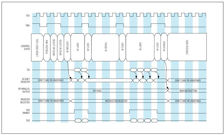
Figure 15-3. TAP Controller Debug Mode IR-Scan Example
