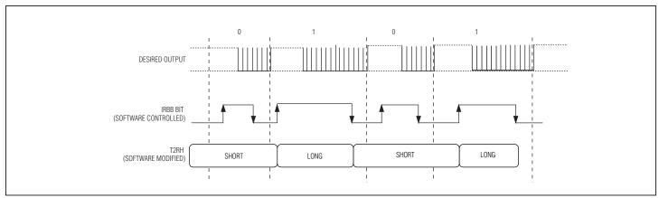
Figure 9-11. Bit-Length Encoding Example (T2RH Modified)
