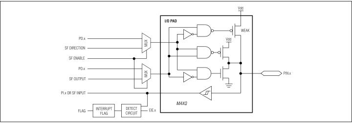
Figure 6-4. Type D Port Pin Schematic
