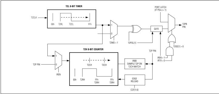
Figure 9-12. IR Receive Pin Sampling
