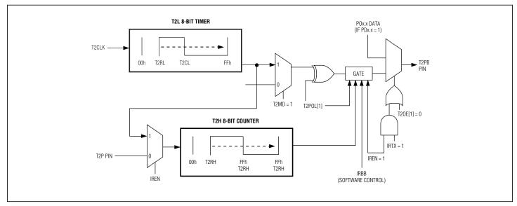
Figure 9-9. IR Transmit Subcarrier Generation and Baseband Modulator Control
