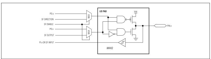
Figure 6-2. Type B Port Pin Schematic
