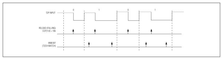
Figure 9-14. Bit Length Decoding Example
