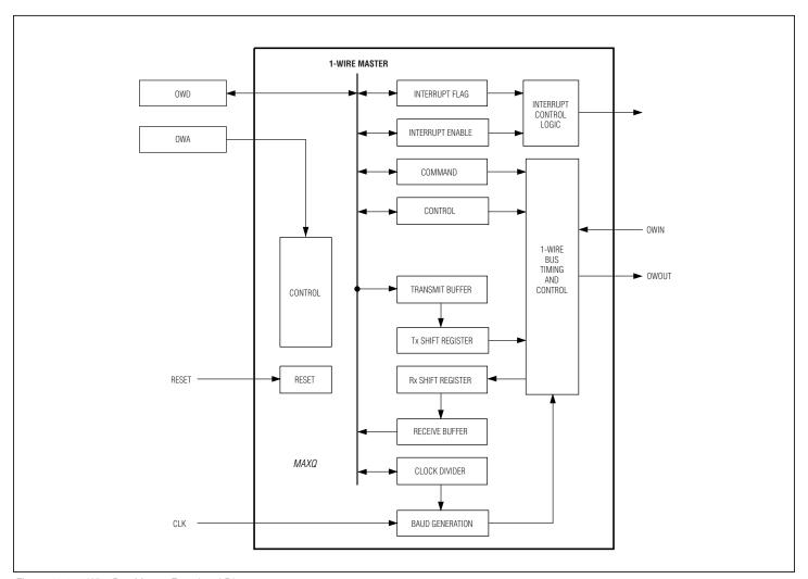
Figure 13-1. 1-Wire Bus Master Functional Diagram
