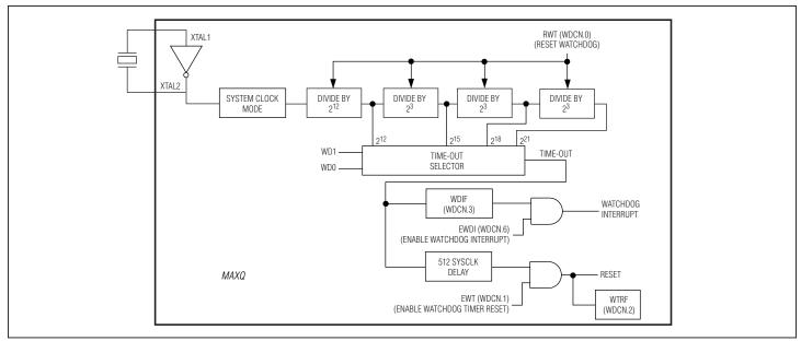
Figure 3-1. Watchdog Timer Block Diagram
