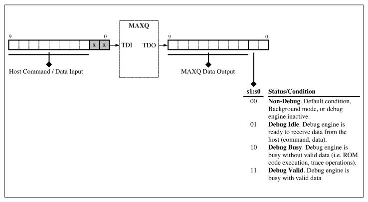
The data byte portion of the 10-bit shift register is interfaced directly to the ICDB parallel register. The ICDB register functions as the holding data register for both transmit and receive operations. On the falling edge of TCK in the Update-DR state, the outgoing data is loaded from the ICDB parallel register to the debug shift register and the incoming shift register data is latched in the ICDB parallel register.
