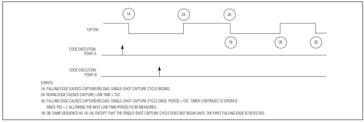
Figure 9-7. Timer 2 Application Example—Measure Duty Cycle
