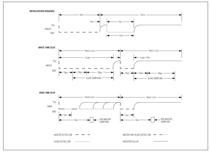
Figure 13-2. 1-Wire Bus Signaling in Standard Mode
