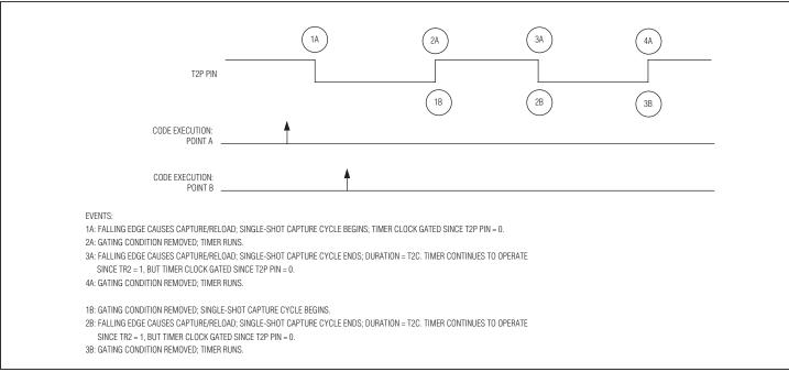
Figure 9-5. Timer 2 Application Example—Measure High Pulse Width
