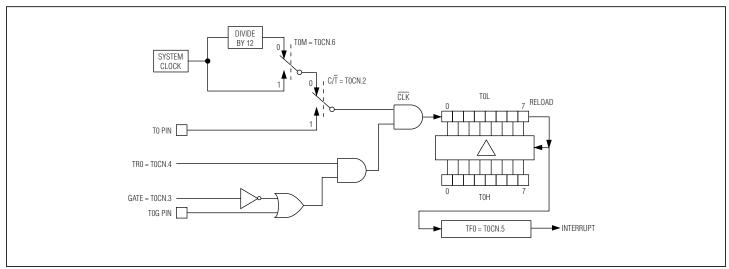
Figure 7-2. Timer/Counter 0 8-Bit Auto-Reload Mode
