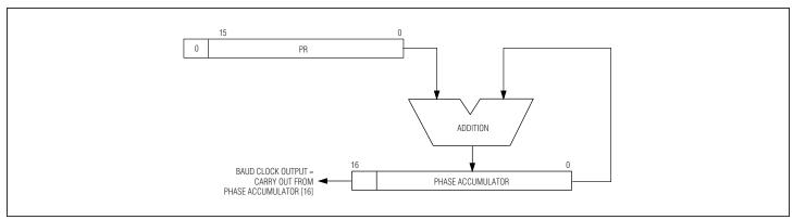
Figure 10-5. Baud-Clock Generator
