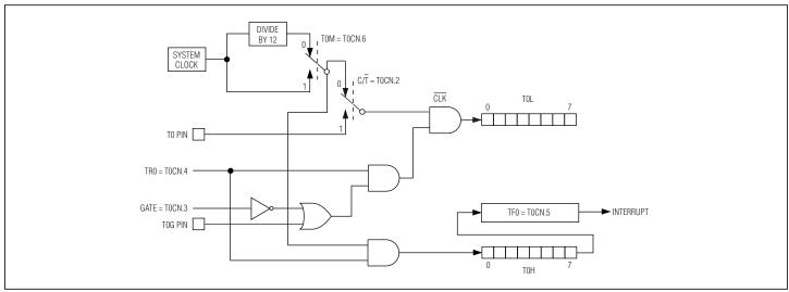
Figure 7-3. Timer/Counter 0 Dual 8-Bit Mode
