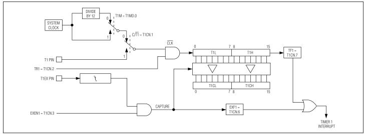
Figure 8-2. Timer/Counter 1 16-Bit Event Capture
