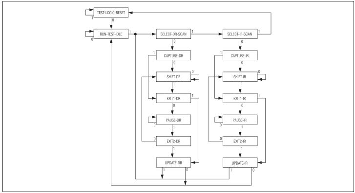
Figure 15-1. TAP Controller State Diagram
