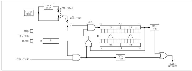
Figure 8-1. Timer/Counter 1 16-Bit Auto-Reload Mode
