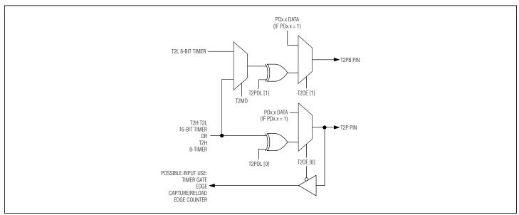
Figure 9-2. Output Enable and Polarity Control
