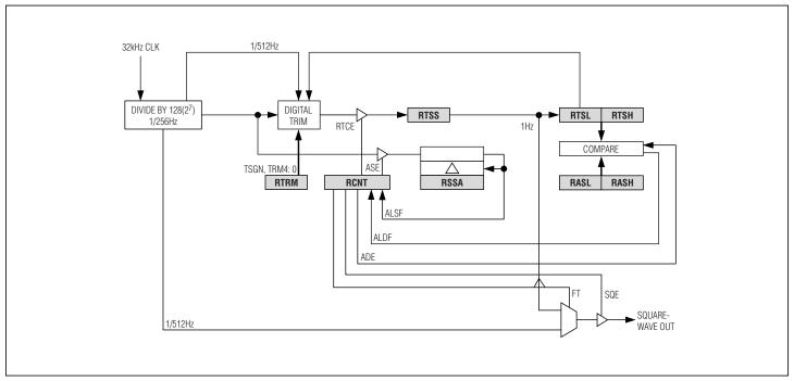
Figure 14-1. RTC Functional Block Diagram
