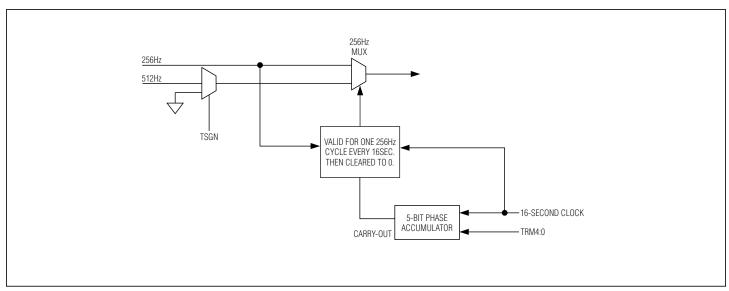
Figure 14-2. RTC Digital-Trim Facility Block Diagram
