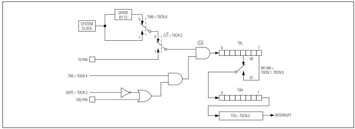
Figure 7-1. Timer/Counter 0 13-Bit/16-Bit Modes
