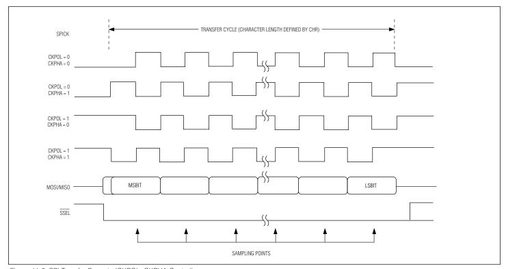
Figure 11-2. SPI Transfer Formats (CKPOL, CKPHA Control)
