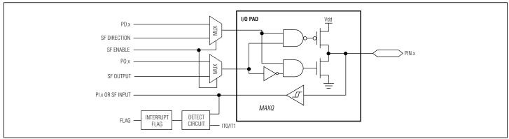
Figure 6-1. Type A Port Pin Schematic
