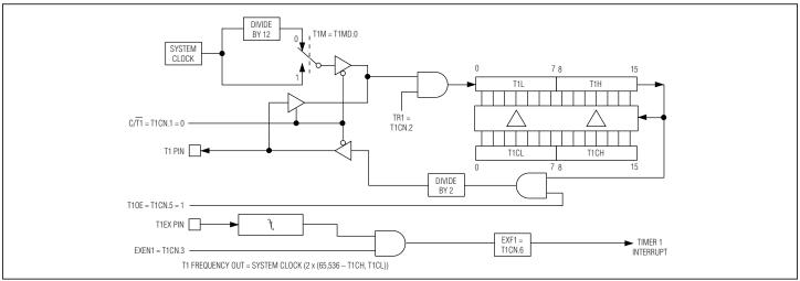
Figure 8-4. Timer 1 Clock Output Mode
