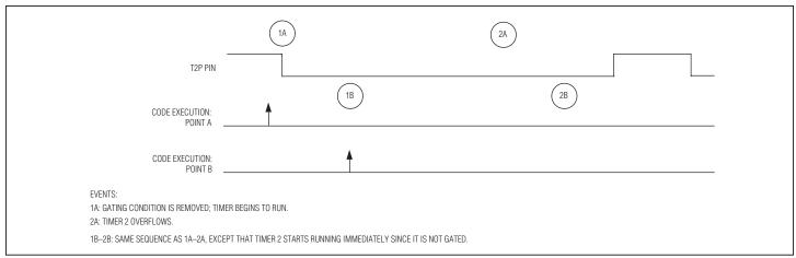
Figure 9-8. Timer 2 Application Example—Overflow/Interrupt on Cumulative Time
