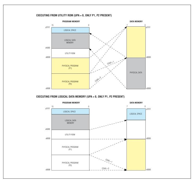
Figure 2-6. CDA Functions (Byte Access Mode)
