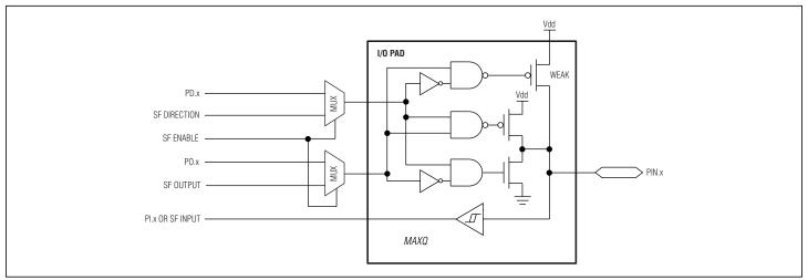
Figure 6-3. Type C Port Pin Schematic
