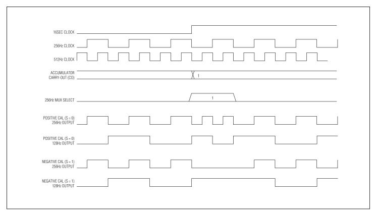
Figure 14-3. Digital Trim Pulse Calibration Diagram
