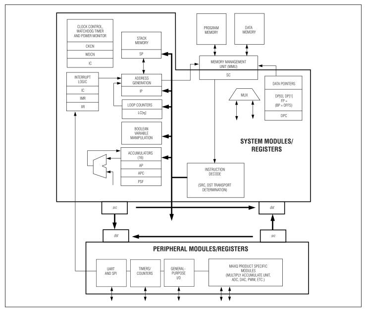
Figure 2-1. MAXQ Transport-Triggered Architecture
