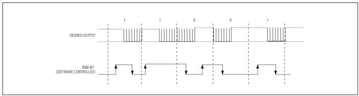
Figure 9-10. Biphase Encoding Example (T2RH Remains Fixed)
