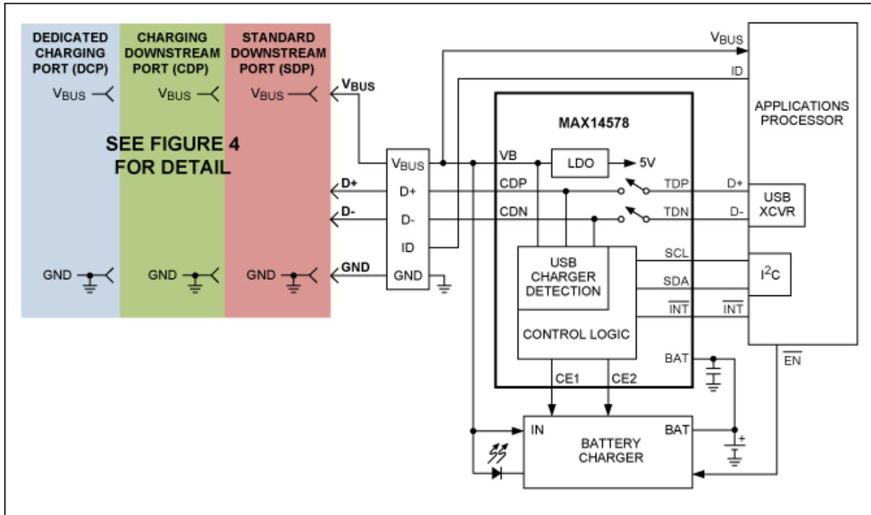
Figure 5. Fully-compliant USB BC1.1 port detection can be added to a charger with the MAX14578 USB charging port detector and data-switch IC.
