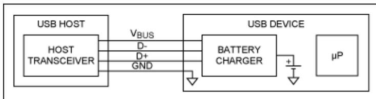
Figure 2. A self-enumerating charger connects directly to the USB data lines, allowing simple systems to fully utilize USB charging without a USB transceiver or microprocessor resources.
