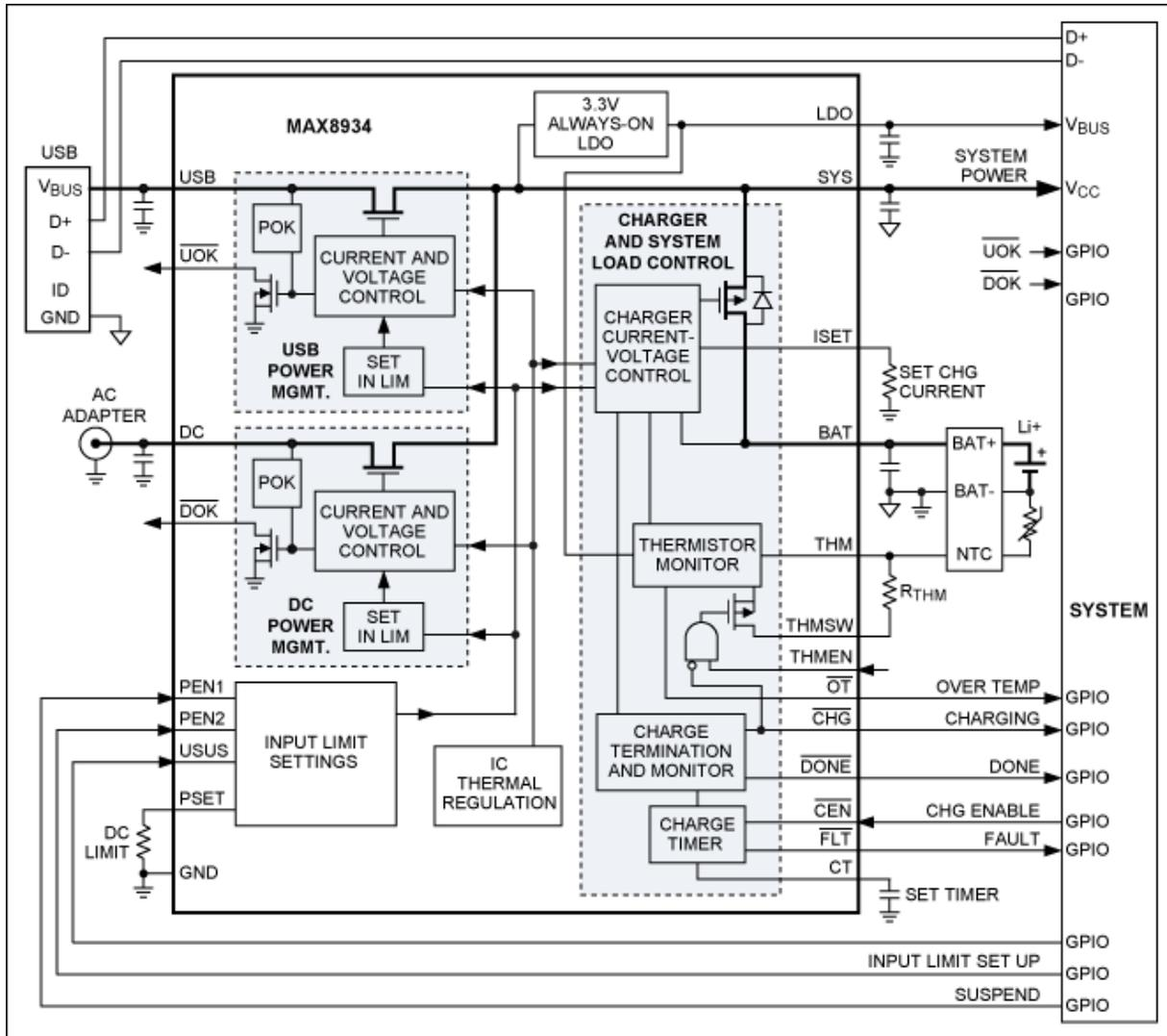
Figure 9. A dual-input USB/adaptor charger with Smart Power Selector functionality like the [MAX8934](#) can power the system immediately when external power is applied while it also charges a dead battery.
