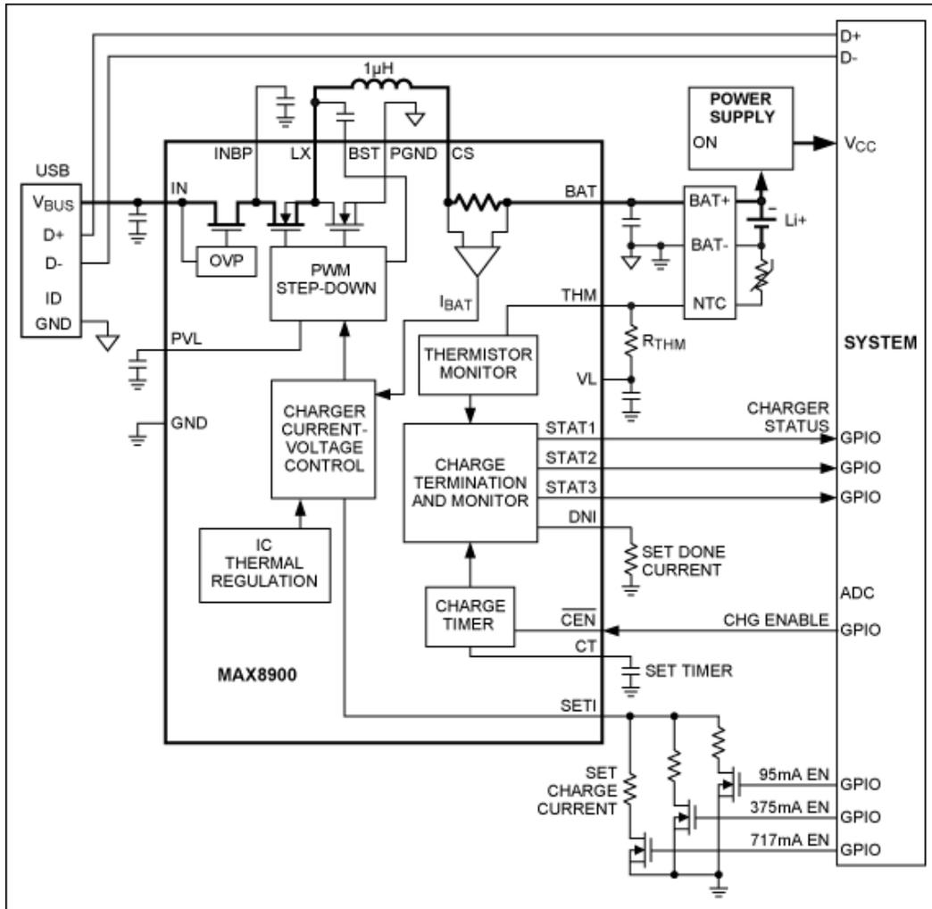
Figure 11. Direct-connect switch-mode charger with  $\pm 22V$  overvoltage and reverse-polarity protection.
