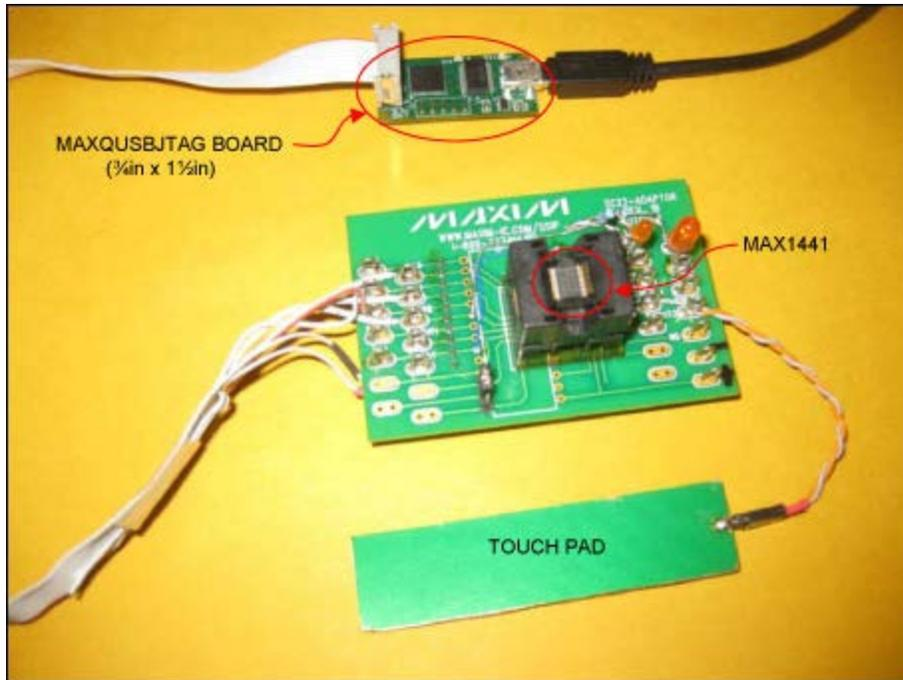
Figure 2. MAX1441 application board and MAXQUSBJTAG-KIT connection setup.
