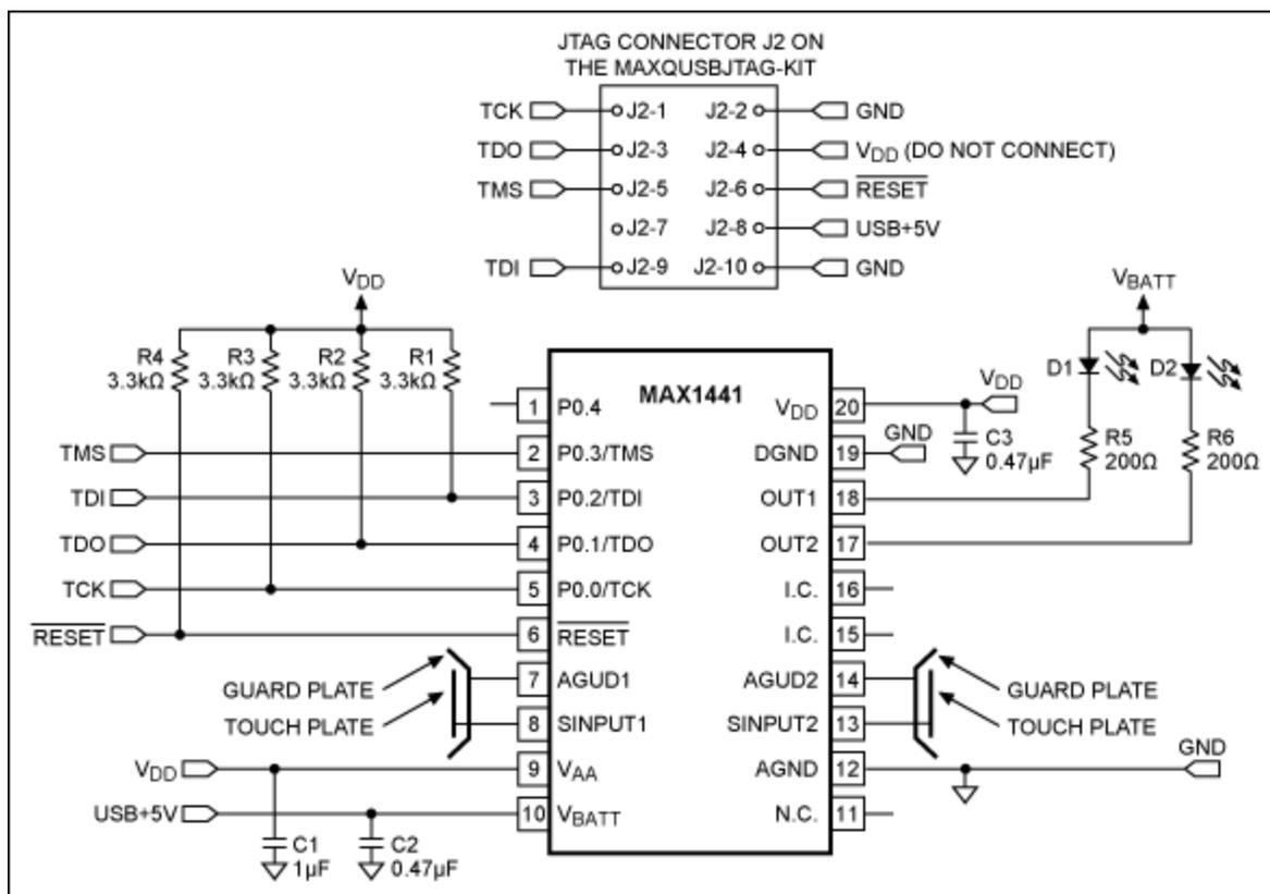
Figure 1. JTAG interface connections between a MAX1441 application circuit and the MAXQUSBJTAG-KIT board.
