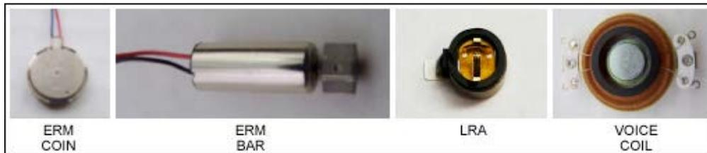
Figure 13. The actuators that were compared and yielded data for Table 2.
