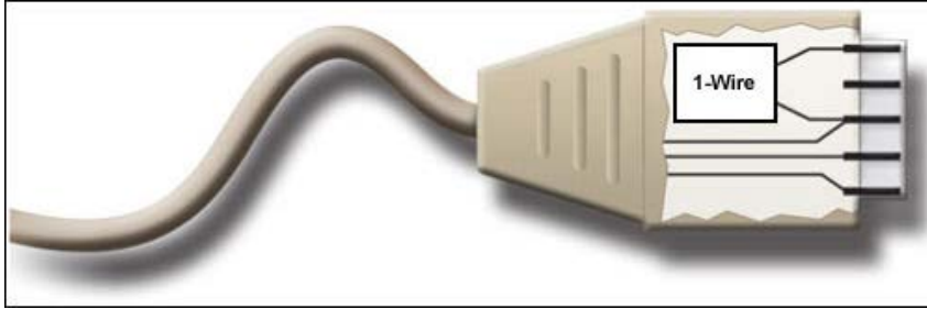
A 1-Wire device and wired sensor with DB9 connector interface to the instrument.
