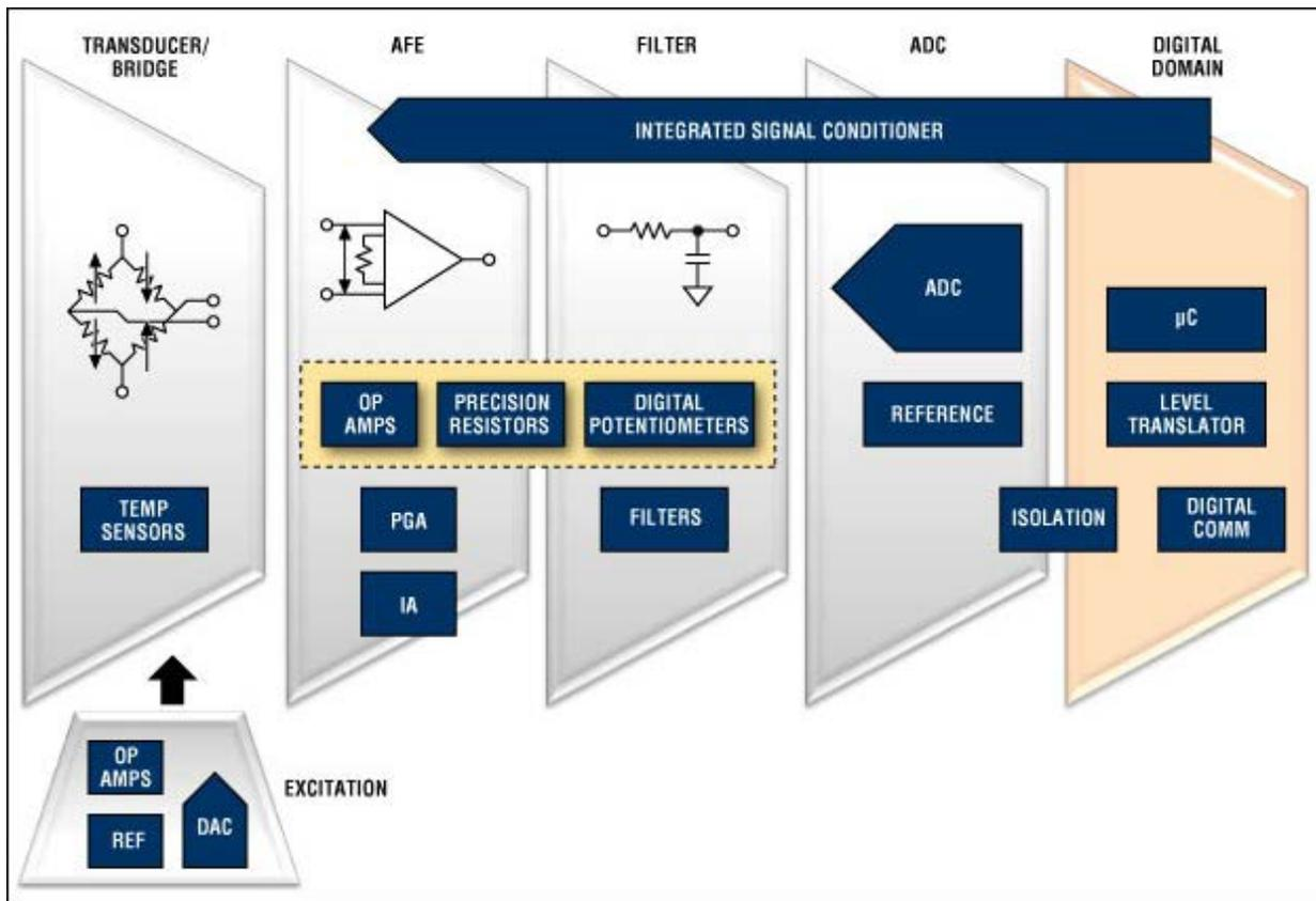
Block diagram of the signal chain in a force-sense application. For a list of Maxim's recommended pressure-sensor solutions, please go to: [www.maximintegrated.com/psi](http://www.maximintegrated.com/psi).
