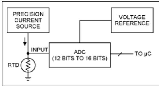
Figure 1. Simplified RTD signal-conditioning circuit.
