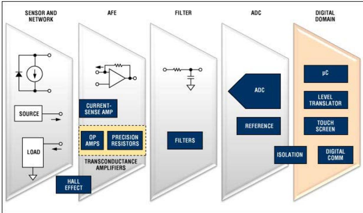
Block diagram of the signal chain in a current-sensing application. For a list of Maxim's recommended current-sensing solutions, please go to: [www.maximintegrated.com/detect](http://www.maximintegrated.com/detect).
