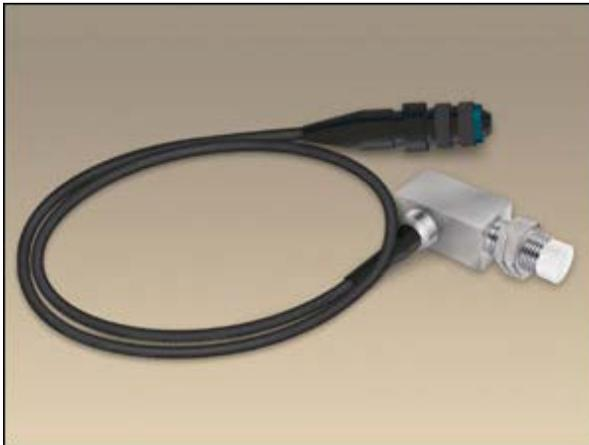
Binary sensors only transmit single-bit information. Typically, the presence or absence of an object is detected and communicated with a logic level. Also, when an object like a piston in a valve reaches a predefined critical distance, the sensor detects and communicates this to the programmable-logic-controller (PLC) system through a binary interface.
