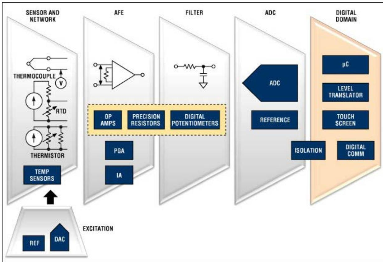
Block diagram of the signal chain in a temperature-sensing application. For a list of Maxim's recommended temperature-sensor solutions, please go to: [www.maximintegrated.com/-40+85](http://www.maximintegrated.com/-40+85).
