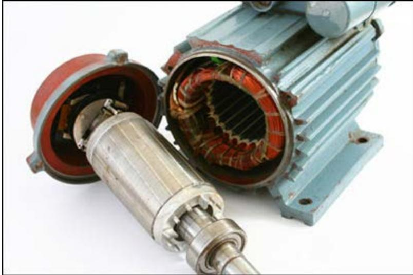
*Rotor and stator of an induction motor.*
