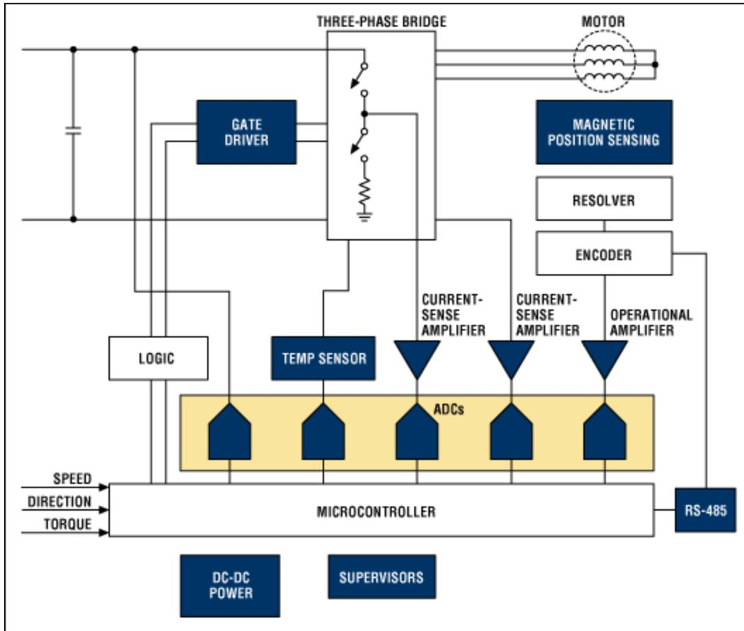
Block diagram of a typical industrial motor control. For a list of Maxim's recommended motor-drive solutions, please go to: [www.maximintegrated.com/motordrive](http://www.maximintegrated.com/motordrive).
