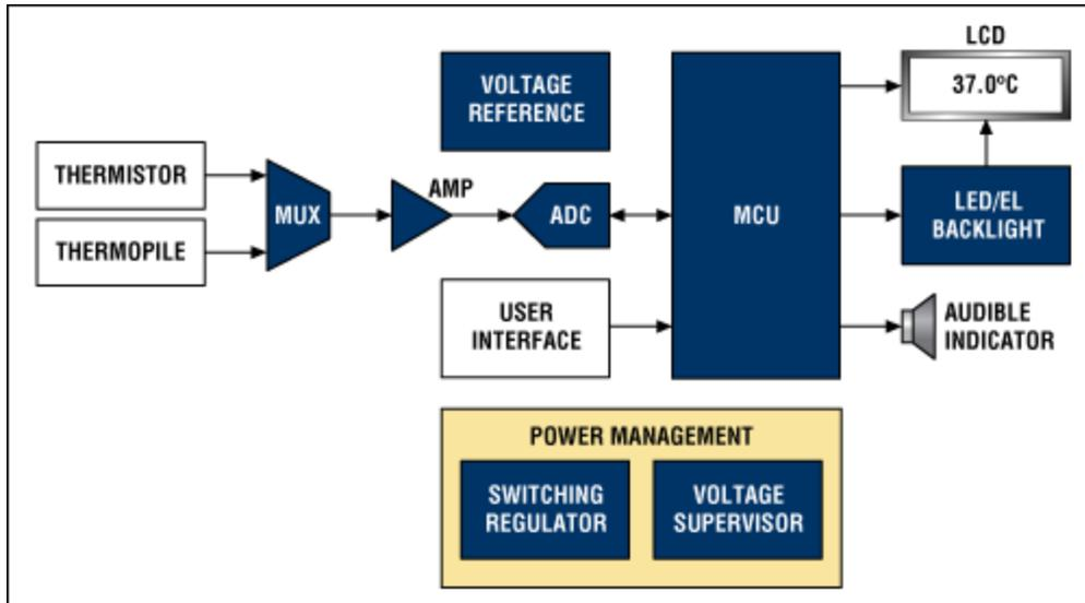
Functional block diagram of a digital thermometer. For a list of Maxim's recommended solutions for digital thermometer designs, please go to: [www.maximintegrated.com/thermometer](http://www.maximintegrated.com/thermometer).
