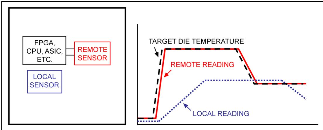
**Figure 17. Comparison of the behavior of a local sensor and a remote sensor. Note that, when an external IC has a thermal diode available, a remote sensor can measure the die temperature of that IC much more quickly and accurately than a local sensor can.**
