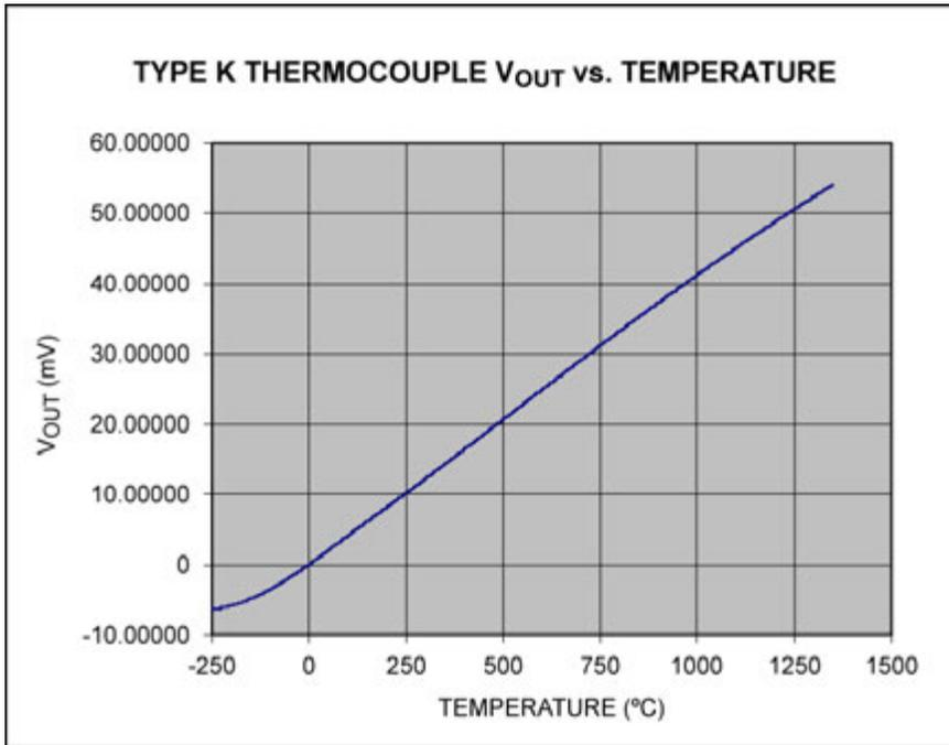
**Figure 7. Type K thermocouple output voltage vs. temperature.**
