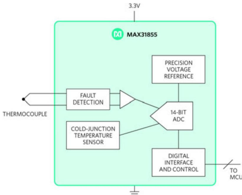
**Figure 33.** MAX31855 integrated thermocouple-to-digital converter with 3-wire interface.
