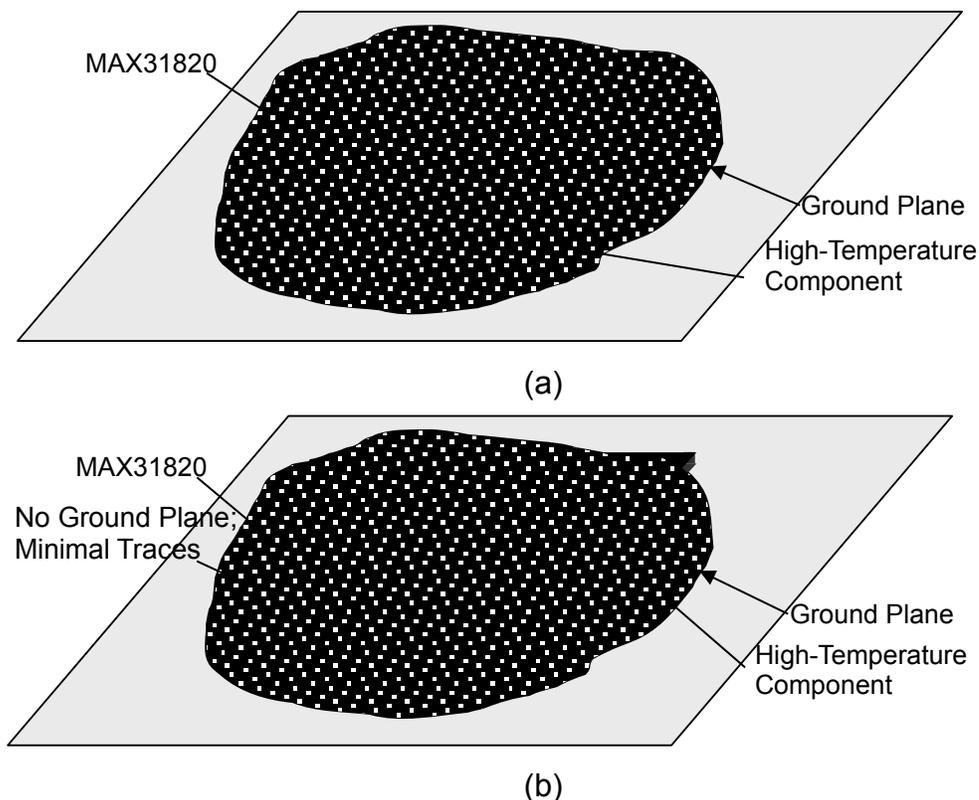
**Figure 36. A board-mounted temperature sensor in a TO92 package. (a) Although the TO92's leads raise the sensor above the board's surface, a high-temperature component and copper nearby can raise the sensor's temperature significantly above ambient. (b) By locating the sensor as far as possible from high-temperature components and eliminating as much copper as possible around the sensor, ambient measurements become more accurate.**
