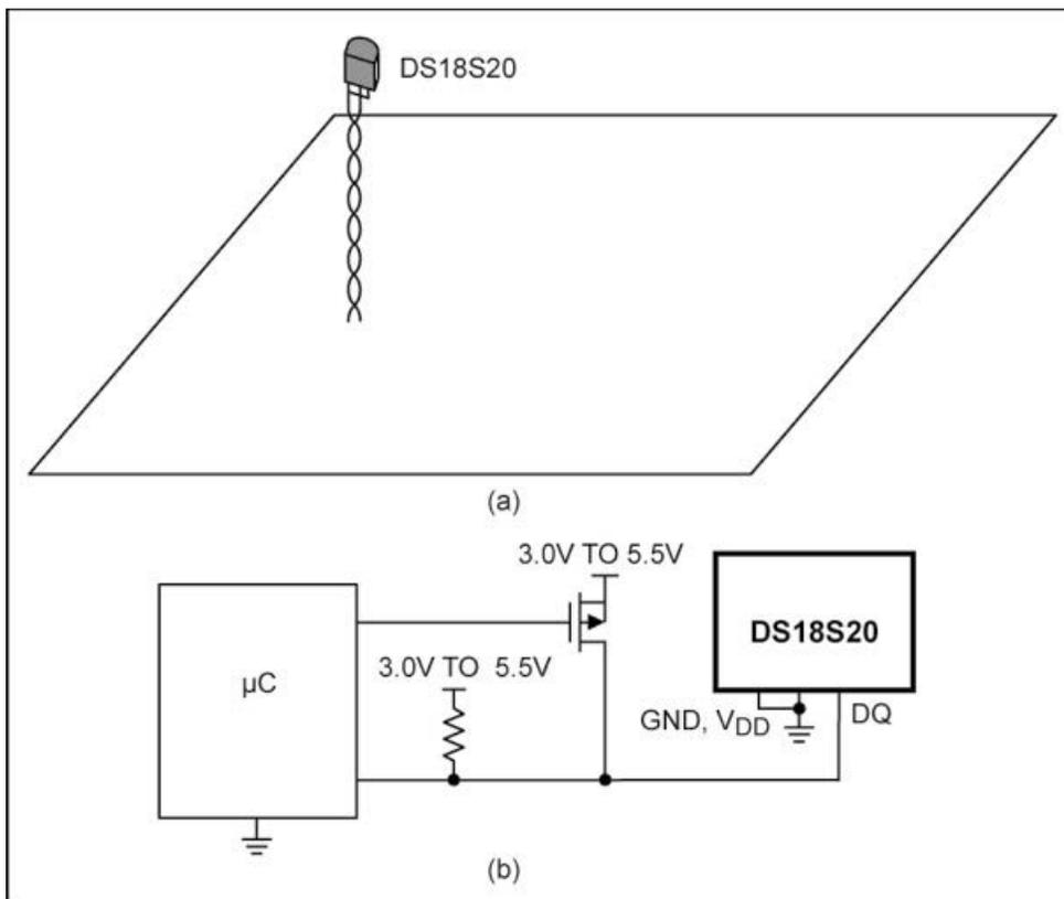
**Figure 37. DS18S20 monitoring ambient temperature. (a) DS18S20 mounted at the end of a twisted pair of wires to isolate the sensor from the PC board. (b) The DS18S20 is powered by the data line. The data and power are controlled by the μC's I/O pins.**
