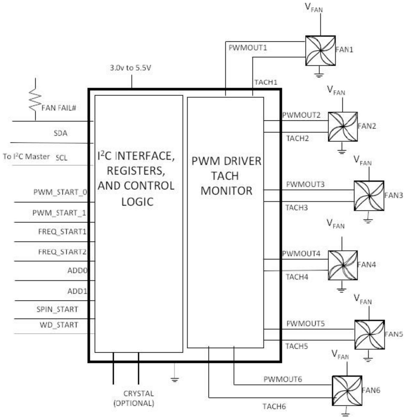
**Figure 50.** If the system microcontroller is capable of monitoring temperature sensors and determining the desired fan speeds, it can communicate the desired speeds to a fan speed
