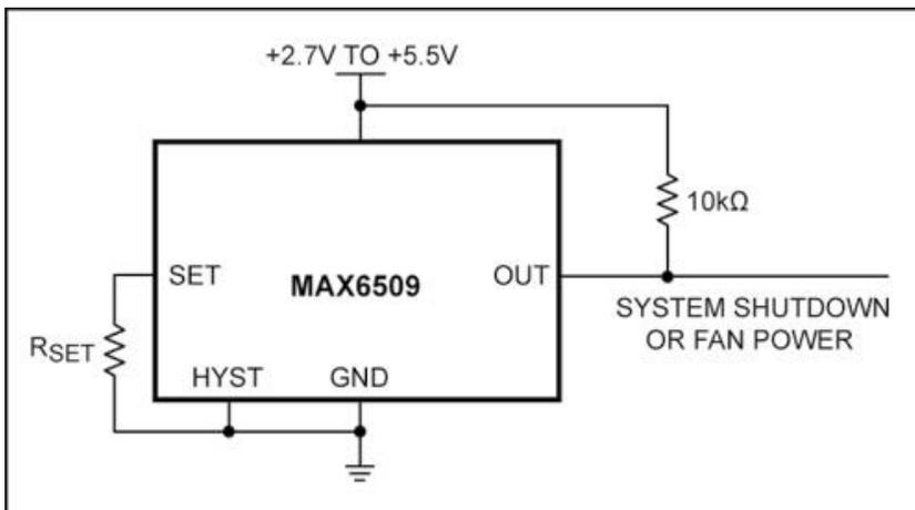
**Figure 20.** Temperature switch with a resistor-set trip temperature.
