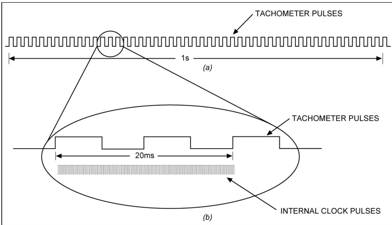
**Figure 26. (a) Monitoring fan speed by counting tachometer pulses for a period of 1s can result in low-resolution measurements. (b) Generating a clock signal with sufficiently high frequency, and then counting the number of clock pulses in a limited number of tachometer periods, provides more resolution and allows the fan’s RPM to be controlled to within a tighter tolerance.**
