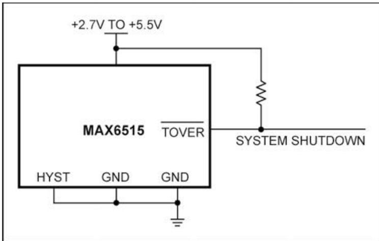
**Figure 19.** Temperature switch with a factory-set trip temperature.
