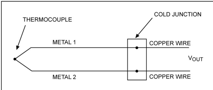
**Figure 9. Simple thermocouple circuit. The junction between metal 1 and metal 2 is the main thermocouple junction. Other thermocouples are present where the metal 1 and metal 2 wires join with the measuring device’s copper wires or PCB traces.**
