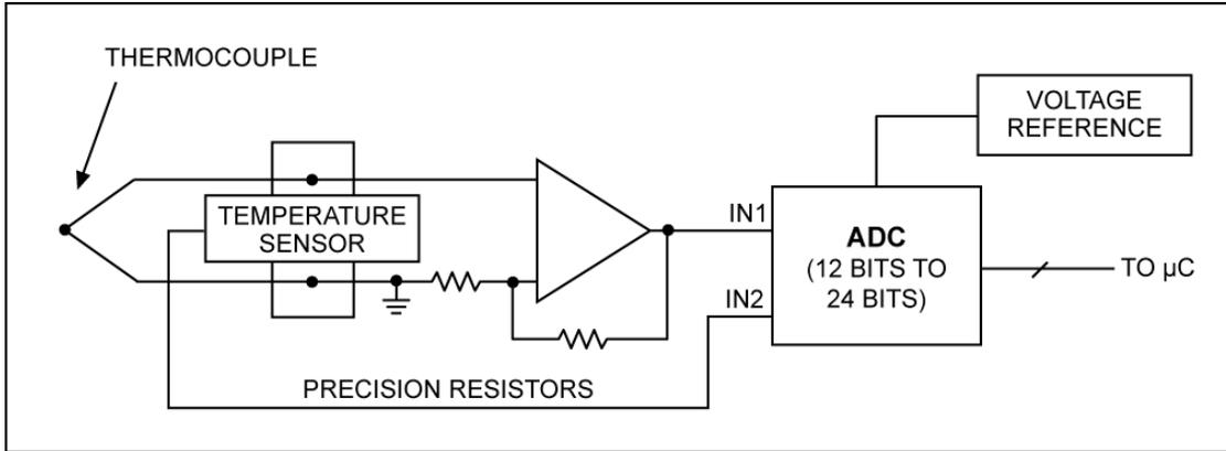
Maxim manufactures ICs (the MAX31850, MAX31851, and MAX31855 series) that perform the signal conditioning functions for a variety of thermocouple types, thus simplifying the design task and significantly reducing the number of components required to amplify, cold-junction compensate, and digitize the thermocouple's output. Thermocouples are available in probes and as elements with bare leads.
