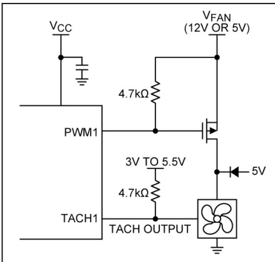
**Figure 29.** A “keep-alive” circuit enables the fan’s tachometer signal even when the PWM waveform is off, thereby avoiding missing tachometer signals while pulse-width modulating the fan’s power supply.
