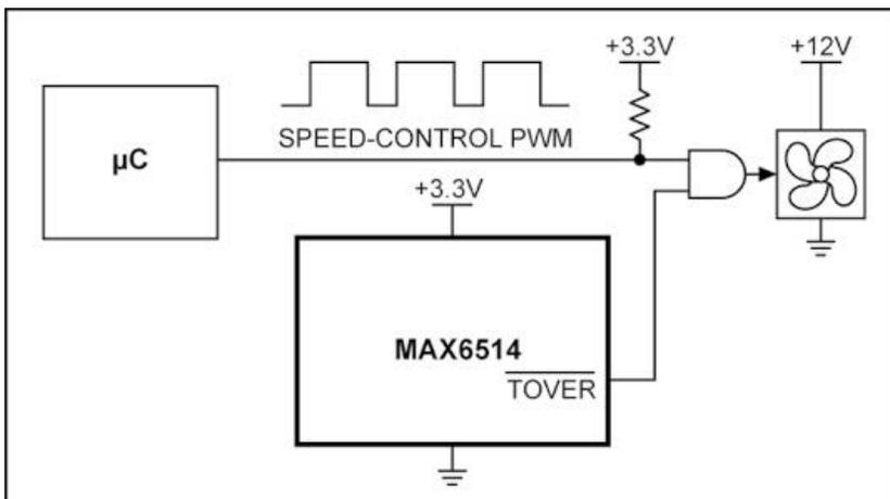
**Figure 65. Fan fail-safe circuit with factory-set trip threshold**
