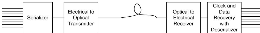
Figure 1. Typical fiber optic link
