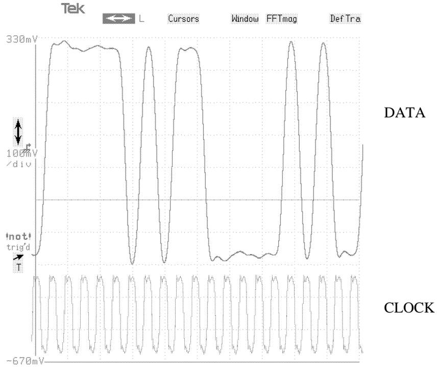
Figure 6. Example using the averaged eye crossing measurement with reduced oscilloscope wander
