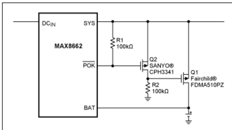
Figure 1. Simplified schematic: reducing  $I^2R$  losses in Smart Power Selector-based battery chargers.
