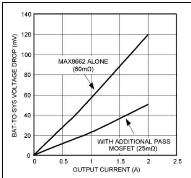
Figure 4. Data for the  $V_{BATT}$ -to- $V_{SYS}$  voltage vs. load current.
