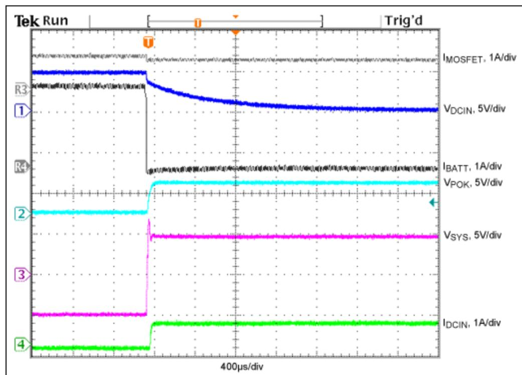
Figure 5. Data show circuit performance when the DC supply is disconnected with  $R1 = R2 = 10k\Omega$ .
