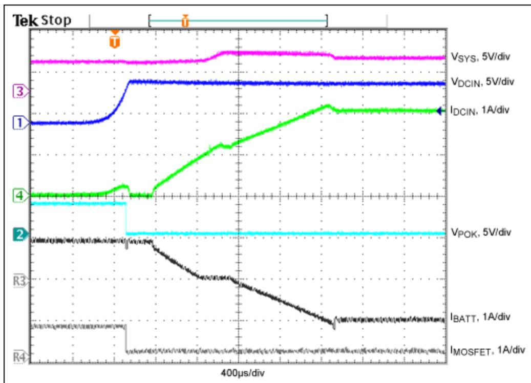
Figure 2. Performance of the Figure 1 circuit when the DC supply is connected.
