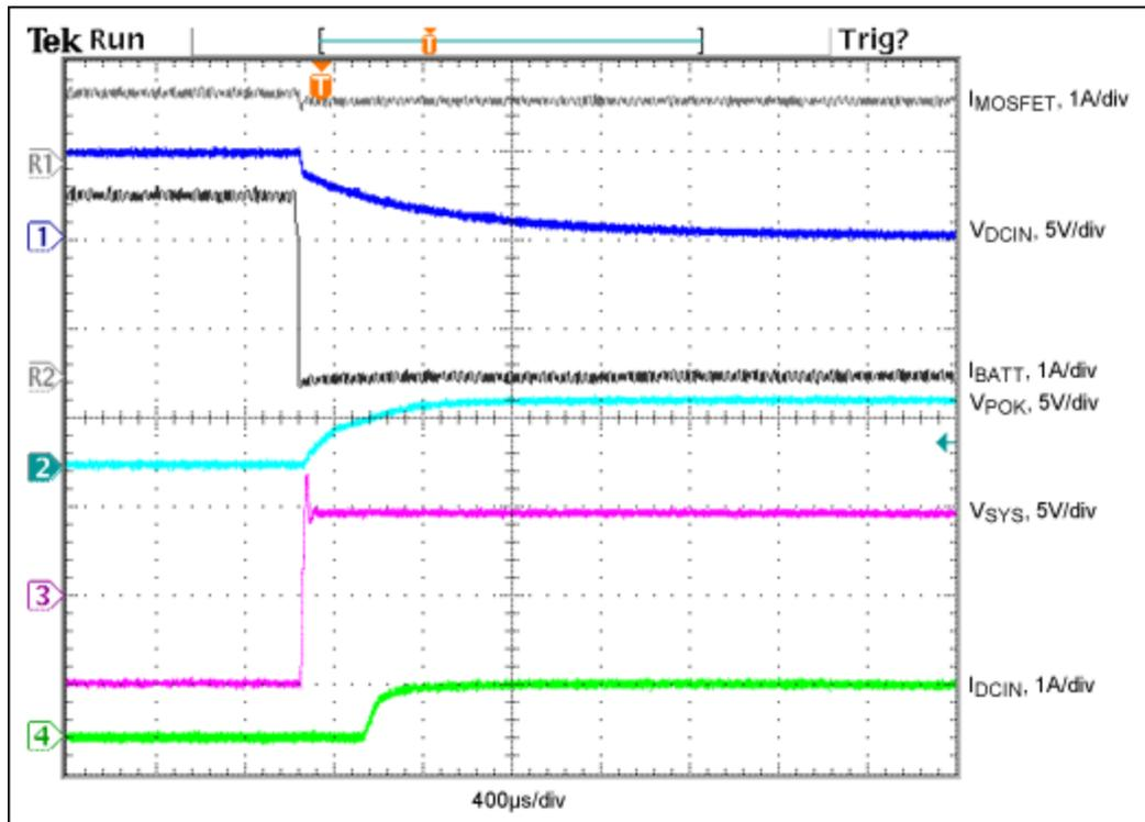
Figure 3. Performance of the Figure 1 circuit when the DC supply is disconnected.
