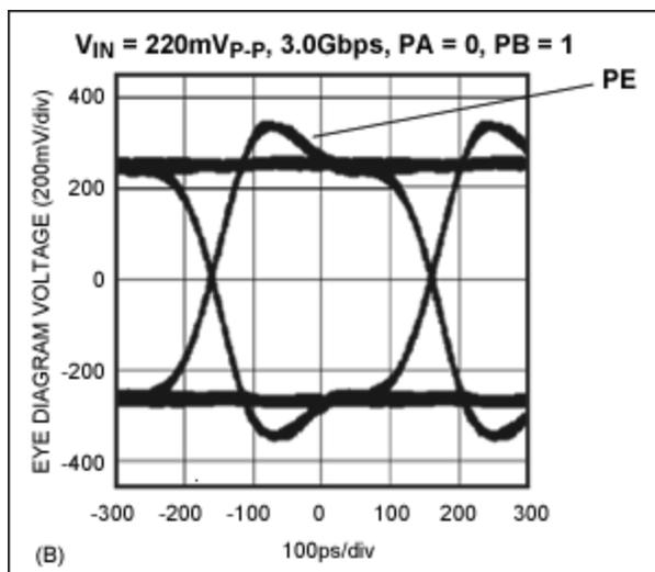
Figure 2B. PE adds amplitude every time that a bit transitions from a 1 to a 0 or a 0 to a 1.
