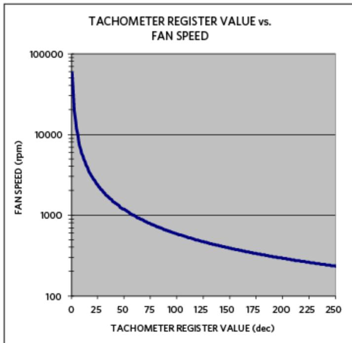
Figure 1. Relationship between tachometer register value and fan speed.
